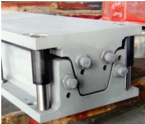
Fig. 95 U-shape steel mold for fabrication of stirrups
