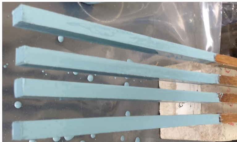
Fig. 103 ExaPhen coating applied on the surface of reinforcements; Left: Without sand particles Right: With sand particles
