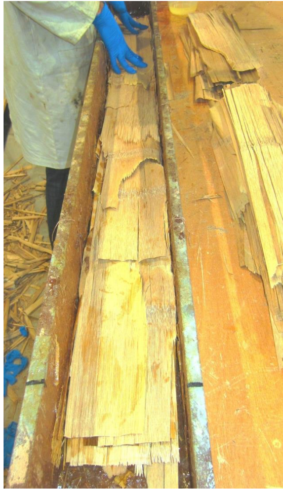
Fig. 93 Hand-layup fabrication for BVC reinforcement
