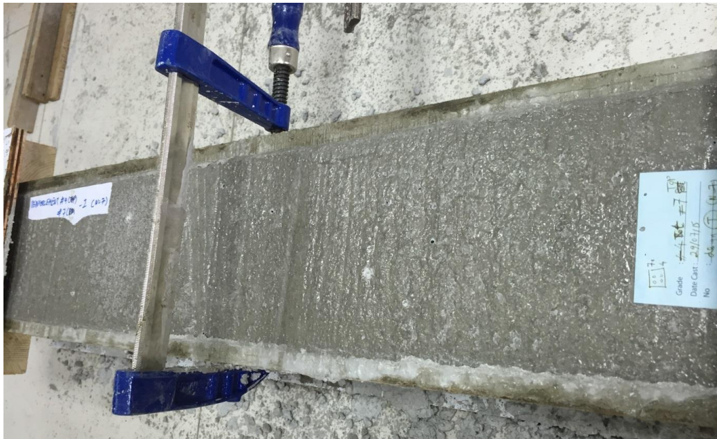
Fig. 155 Final concrete beam prepared with coated BVC reinforcement
