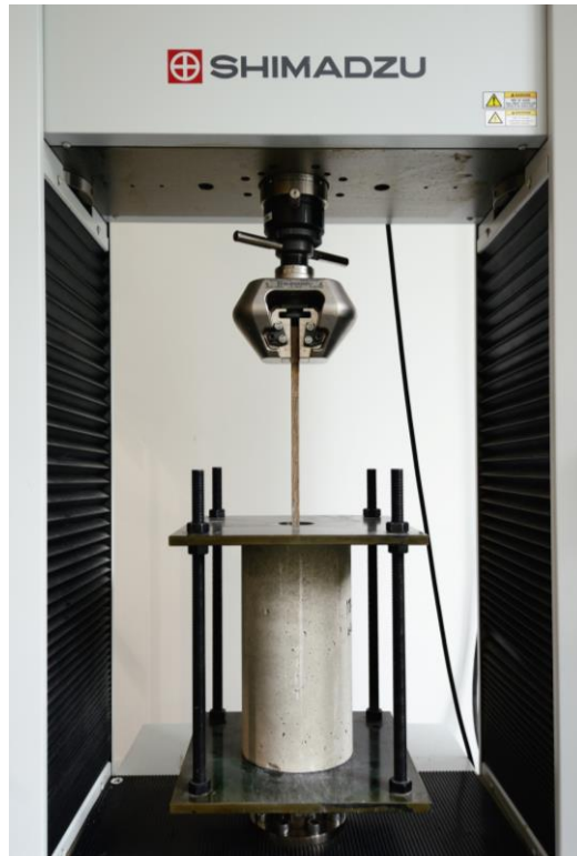
Fig. 109 Pull-out test set-up
