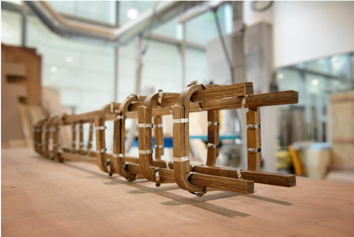
Fig. 151 The BVC reinforcement systems prepared for the concrete beams before applying the coating
