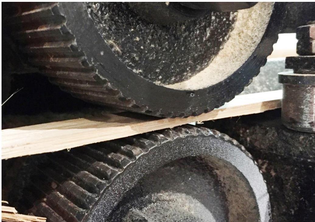
Fig. 89 The metal wheels with ribs used during the bamboo strand processing
