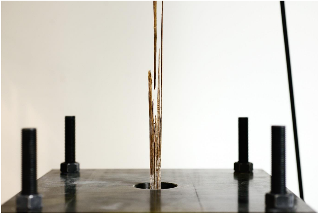
Fig. 116 Tensile rupture of the BVC bar during the pull-out test
