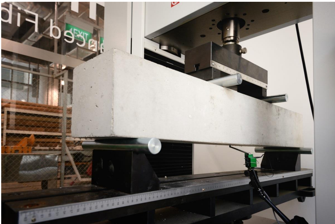
Fig. 159 Concrete beam under four-point flexural test set-up at AFCL Singapore
