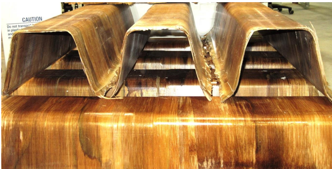
Fig. 97 BVC stirrup samples after removal from the curing oven before cutting into required width
