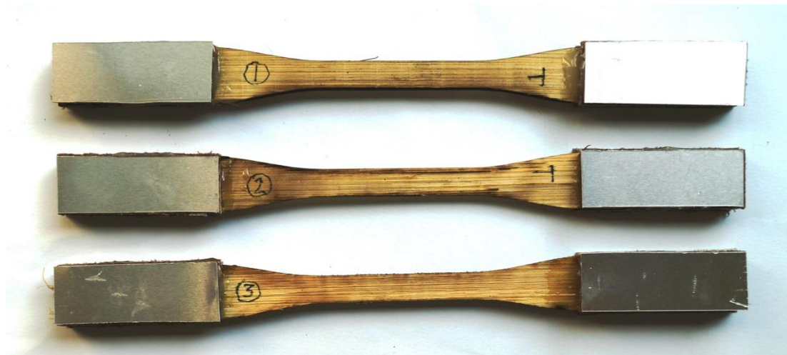
Fig. 50 Tensile test samples from raw bamboo sections
