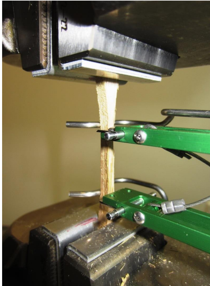
Fig. 52 Modulus of elasticity measurement with extensometer attached to the gauge length of dog-bone samples
