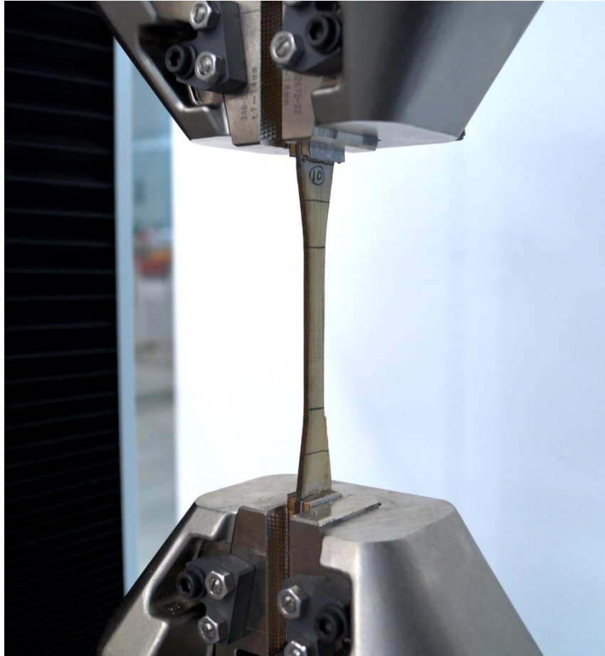
Fig. 51 Bamboo tensile samples under UTM machine for testing
