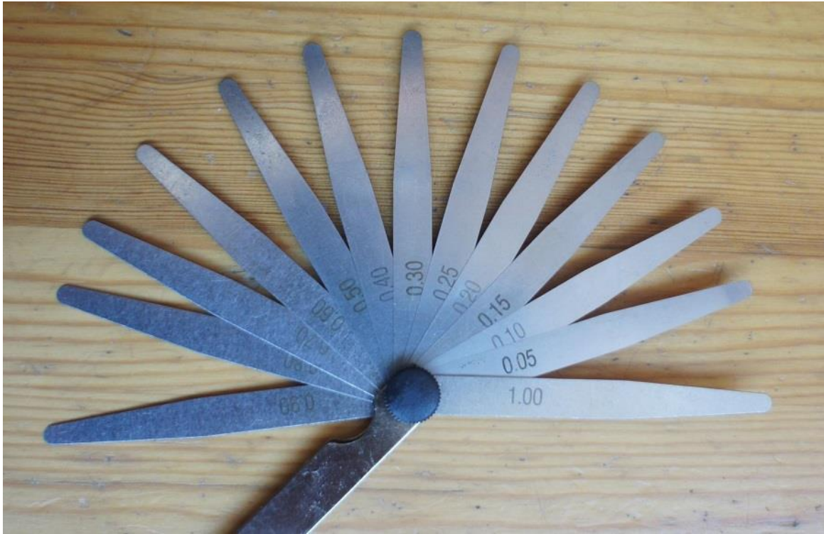
Fig. 158 Feeler gage used for measuring the gaps between concrete surface and the rollers
