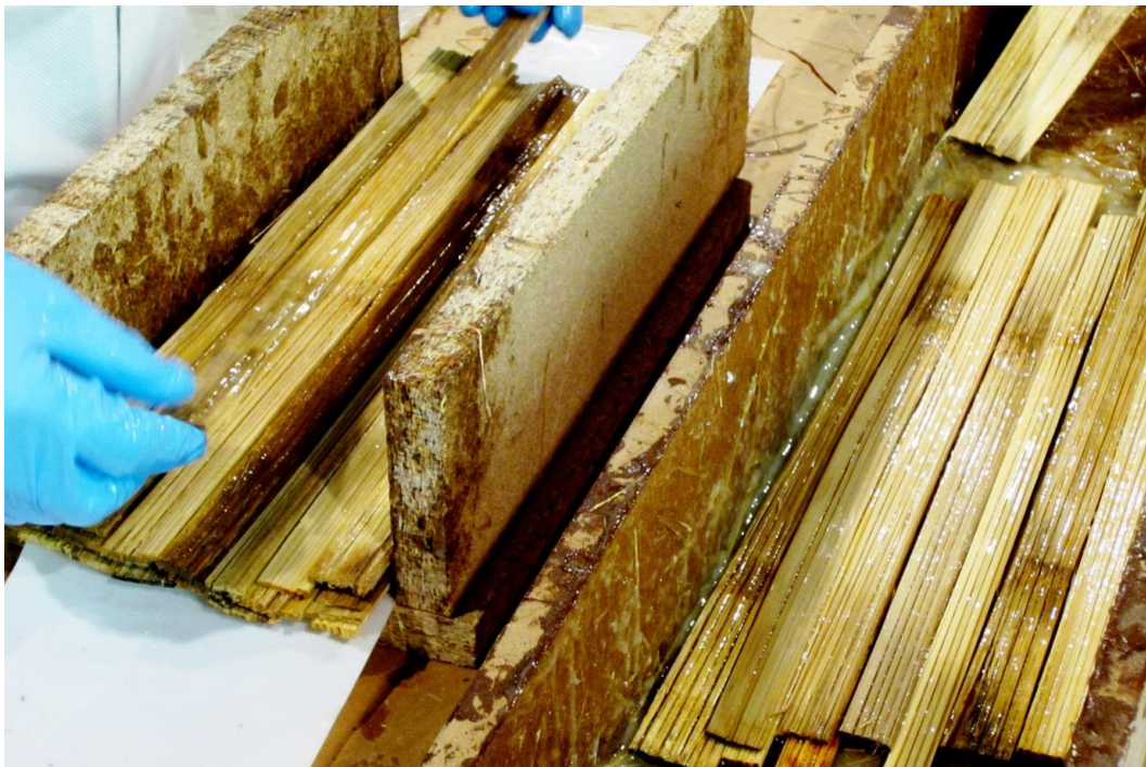
Fig. 69 Hand lay-up process for composite fabrication
