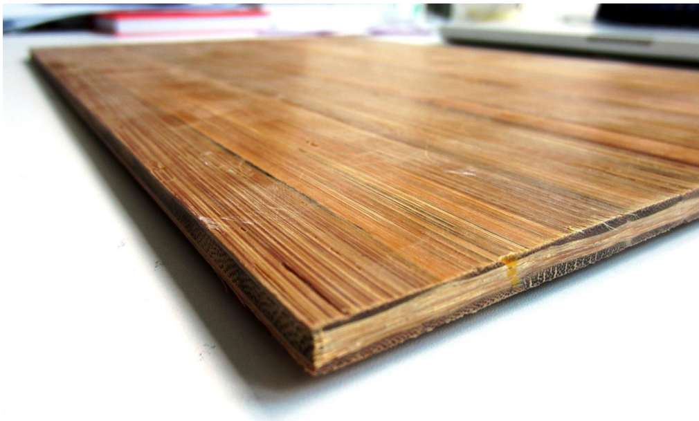
Fig. 70 Bamboo strand composite board after pressing
