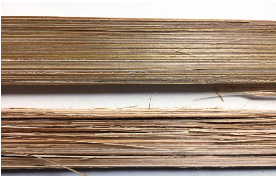
Fig. 61 Bamboo strips before (top) and after (bottom) stranding process
