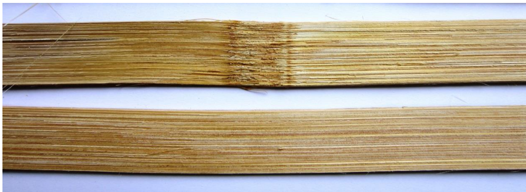
Fig. 58 Bamboo slats after removal of waxy skin and inner nodes
