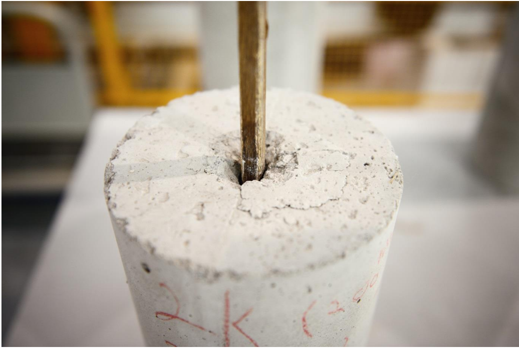
Fig. 114 Bond failure and slippage of BVC bar from the concrete matrix
