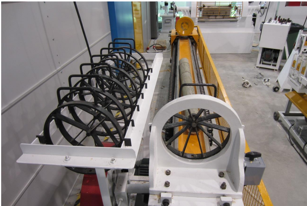
Fig. 56 Bamboo splitting machine at AFCL
