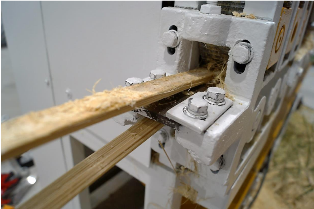
Fig. 49 Thick split culm sections were further split into two equivalent pieces for testing
