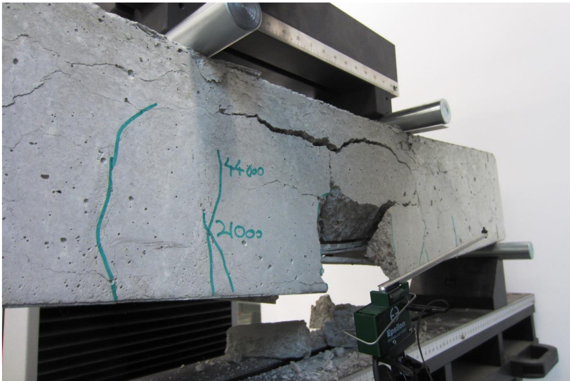
Fig. 168 Concrete crushing mode of failure
