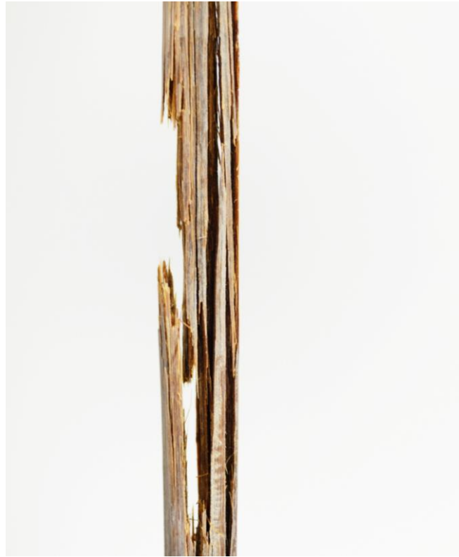
Fig. 118 Tensile failure of the BVC bar
