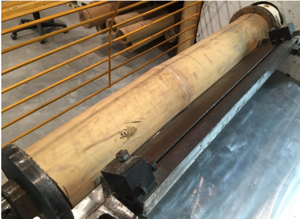
Fig. 63 Bamboo section fixed to the set-up of a peeling machine
