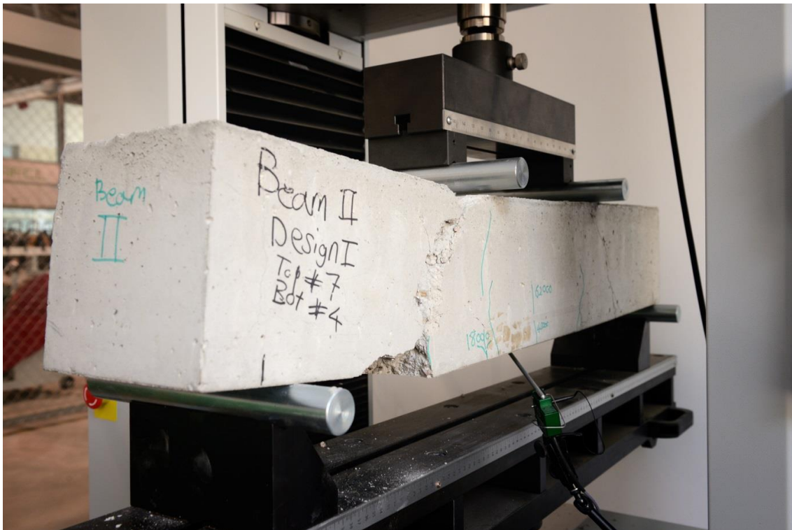
Fig. 161 Shear failure of concrete beam from B1b2 series
