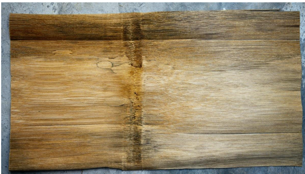
Fig. 67 Bamboo veneers with horizontal lines due to presence of knots
