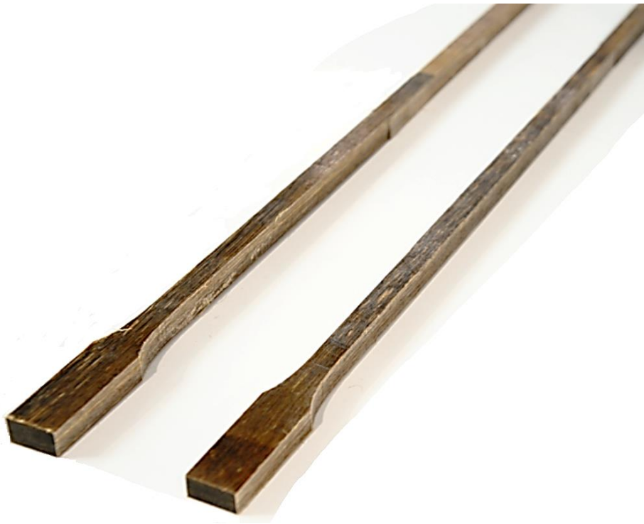
Fig. 101 BVC pull-out samples with dog-bone shaped grip
