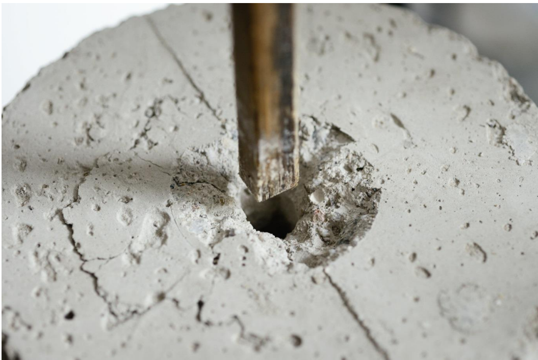
Fig. 115 Complete pull-out of BVC bar from the concrete cylinder due to bond failure
