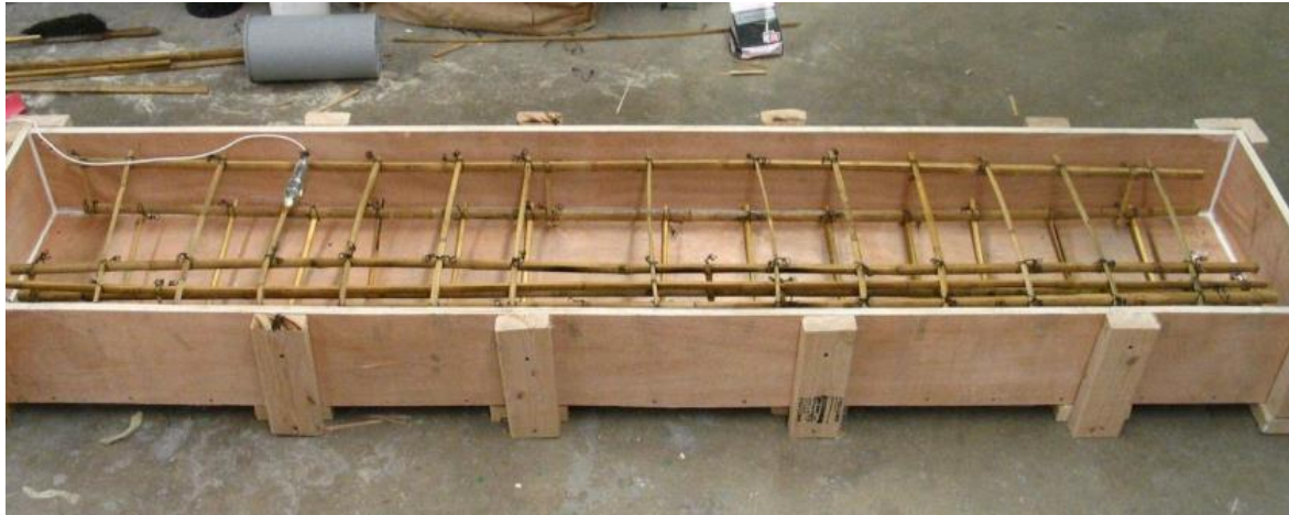
Fig. 44 Bamboo reinforcement and stirrups used to reinforce concrete beam of up to 2.5m in length (Khare 2005)
