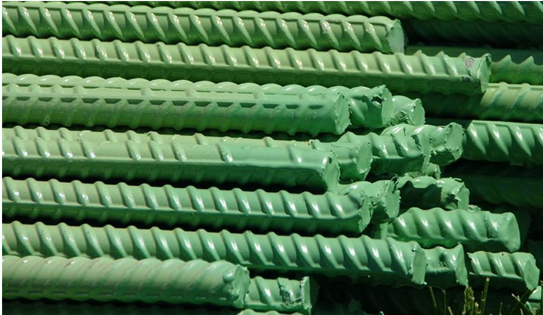
Fig. 20 Epoxy Coated Reinforcement (ECR) bars (National Precast Concrete Association 2015)
