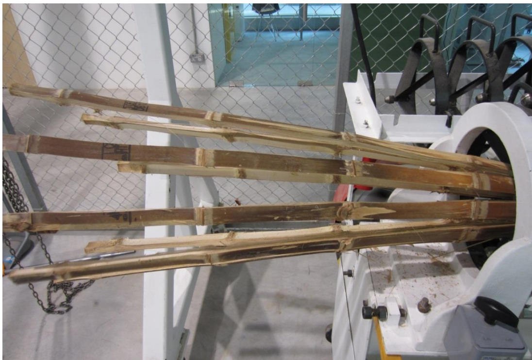
Fig. 48 Splitting the bamboo culms into sections for testing
