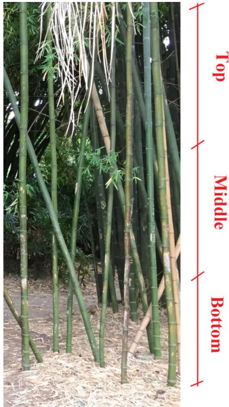
Fig. 47 Top, middle and bottom section definitions of a typical bamboo culm used in this research
