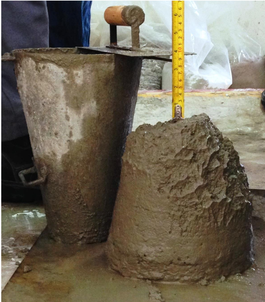
Fig. 106 Slump test procedure to monitor the consistency between various concrete batches
