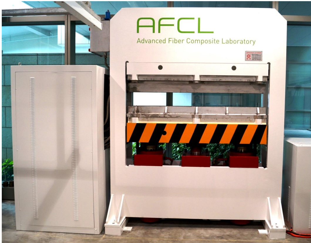
Fig. 68 Hot-press compression molding machine at AFCL Singapore
