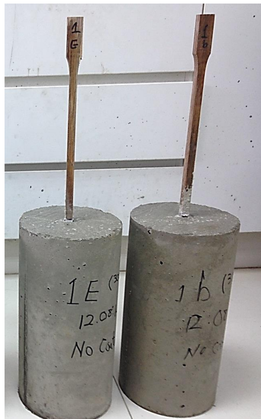
Fig. 107 Details of the pull-out concrete sample with embedment BVC bar
