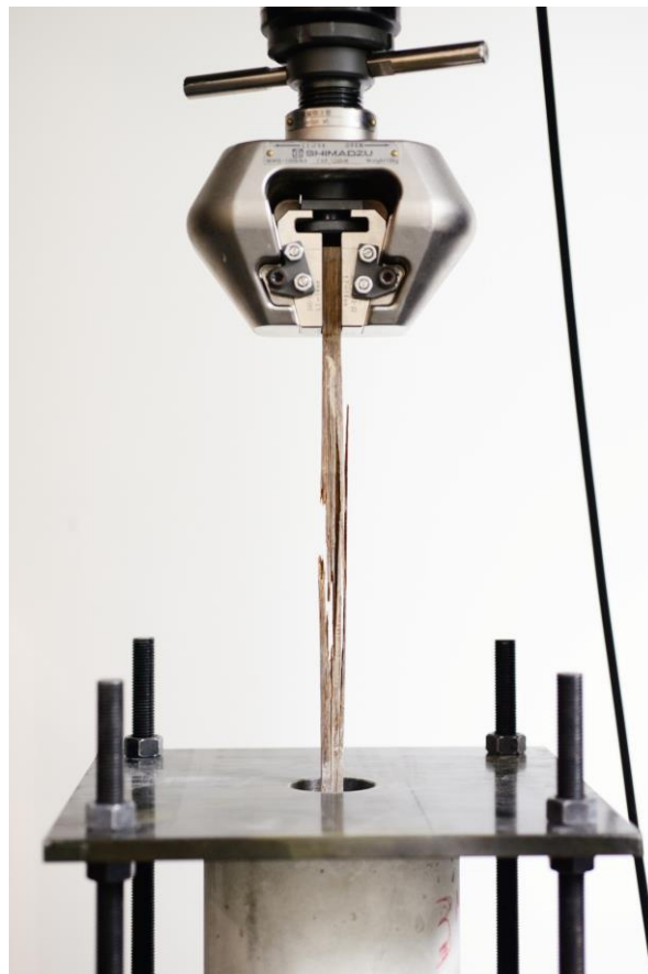
Fig. 117 Tensile failure of the BVC bar tested under the UTM machine
