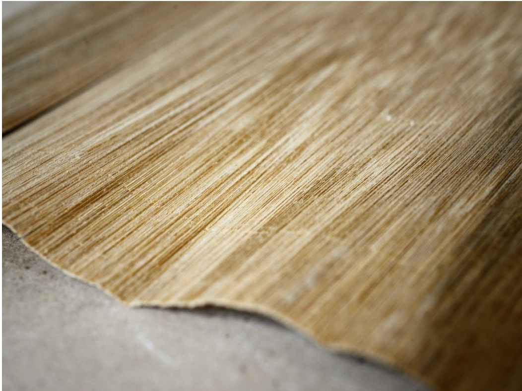
Fig. 66 Bamboo veneers without any knots in between
