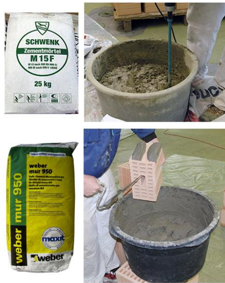
Figure 3-8. Mortar used for the construction of the specimens
