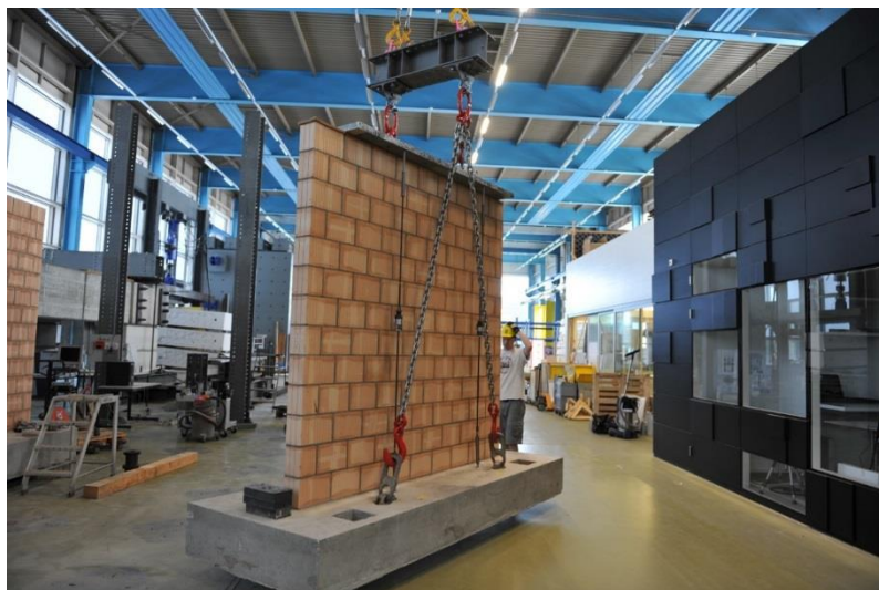
Figure 3-4. Transferring the specimens into the test set-up
