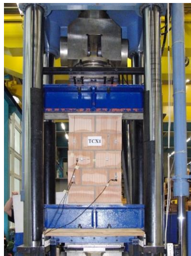
Figure 3-12. Test set-up for the compression tests in the main phase
