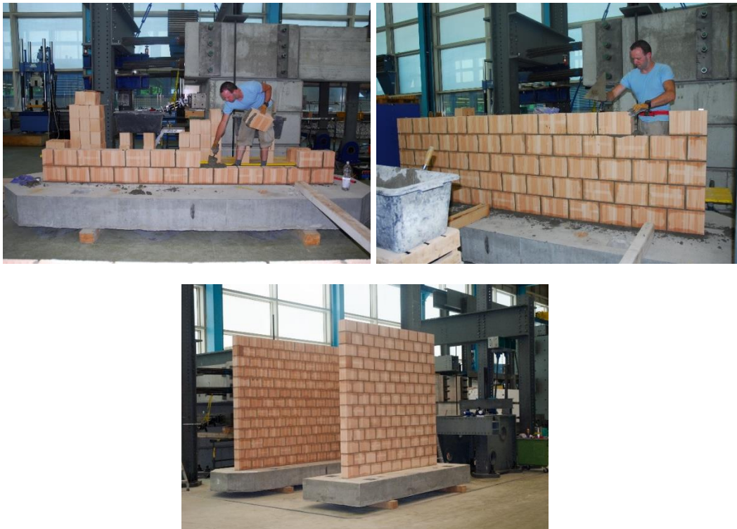
Figure 3-1. Construction of the specimens
