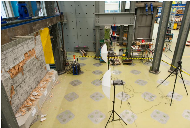
Figure C-1. Implemented 2D DIC measurement system
