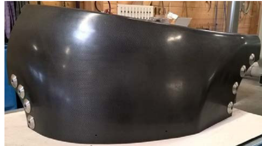
Fig. 14. CFRP structural part for highly-dynamic multiaxial testing machine with optimized inserts.
