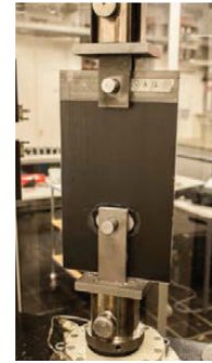
Fig. 5. CFRP sample with insert during the pull-out test.
