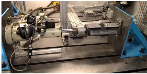
Fig. 13. Fatigue testing in the hydropulser machine.
