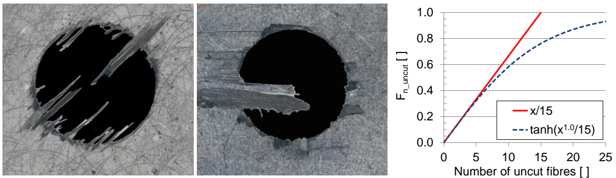
Figure 6.1: Bore exit in CFRP ( \varnothing 6.35 mm) with numerous fine (left) and single wide uncut fibre bundle (middle) and plotted hyperbolic tangent for F_n (right); published in [234]
