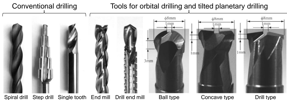
Figure 2.18: Tool geometries for conventional drilling of CFRP in contrast to orbital and tilted planetary drilling, according to [13, 215]
