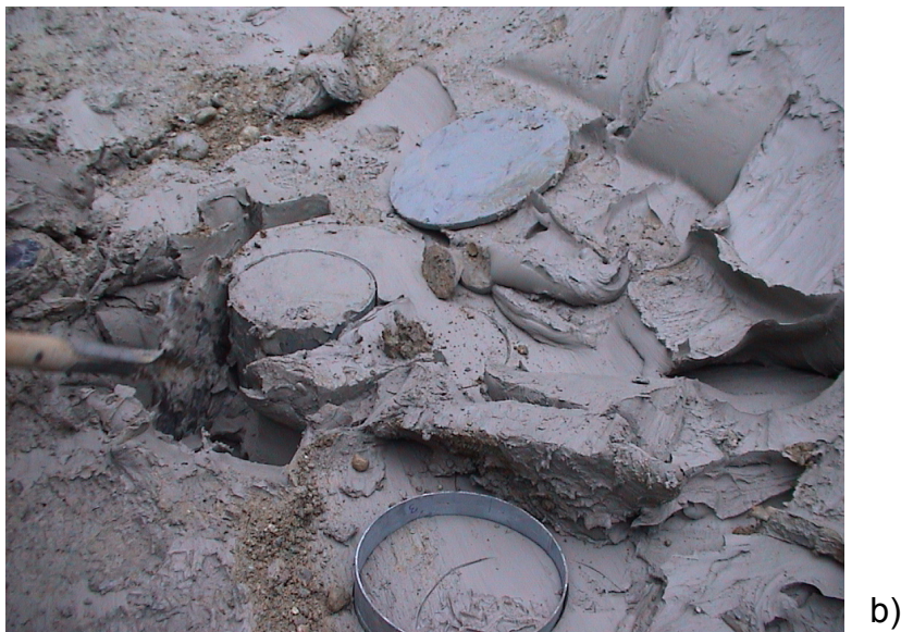
Fig. 3.7: a) Sample tubes pressed into the soil at the bottom of the trench; b) excavating the sample tubes in the trench.
