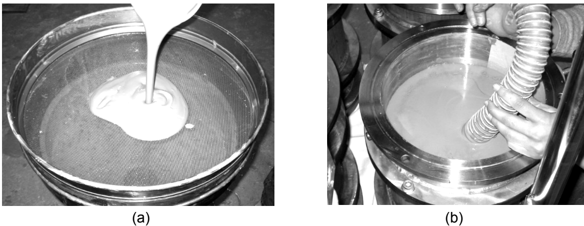
Fig. 3.8: Reconstituted sample preparation: a) sieving the slurry; b) filling the slurry into an oedometer tube.
