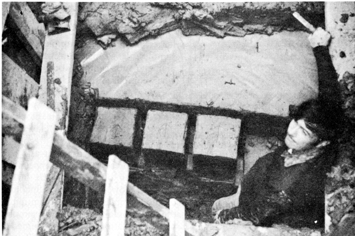
Fig. 2.9: Carving of block samples at the bottom of an opened trench (Lefebvre & Poulin, 1979).
