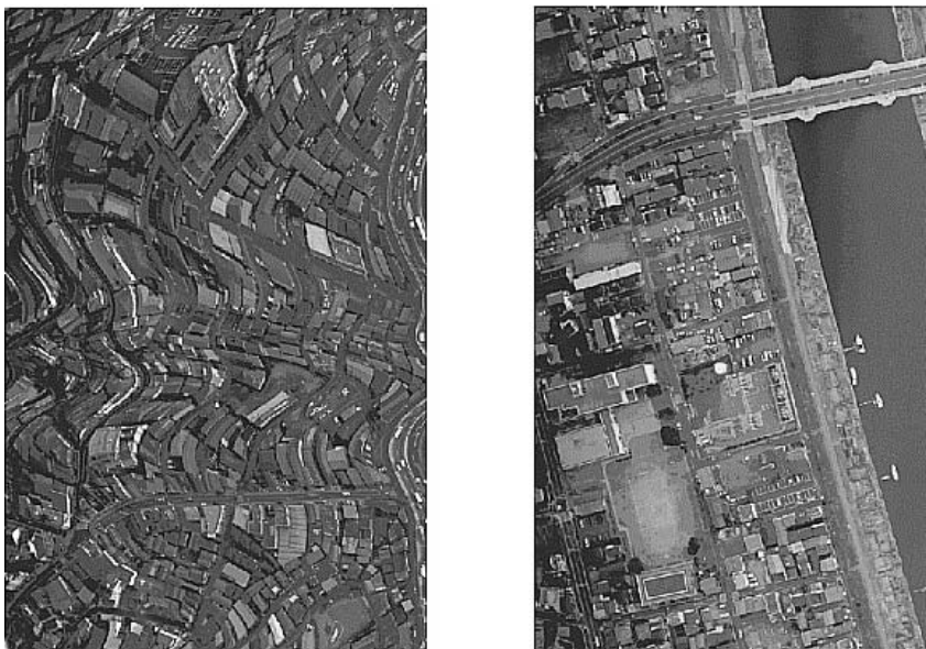
Figure 2.8. Parts of images acquired with the aerial STARIMAGER sensor, without (left) and with (right) gyro-stabilizer (Tsuno et al., 2004).
