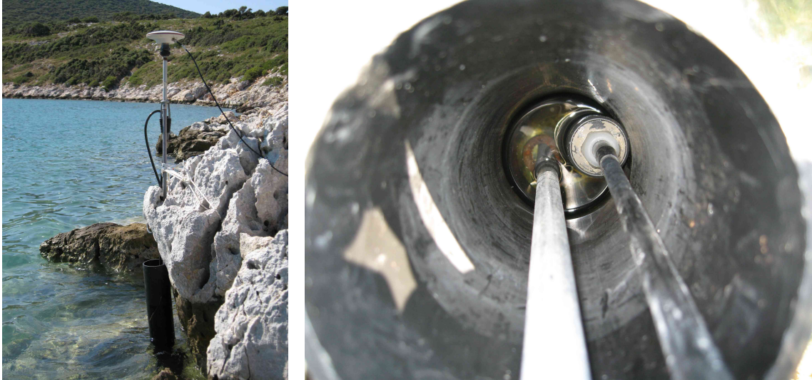
Figure 9.6: Left: Pressure tide-gauge station PELAN, with GPS antenna for the determination of absolute height and position. Right: view of the pressure gauge inside the black tube.
