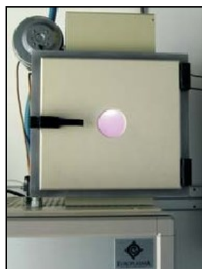
Figure 1.11: DEAEPN and the use of a low pressure radio frequency plasma reactor for the PIGP process
