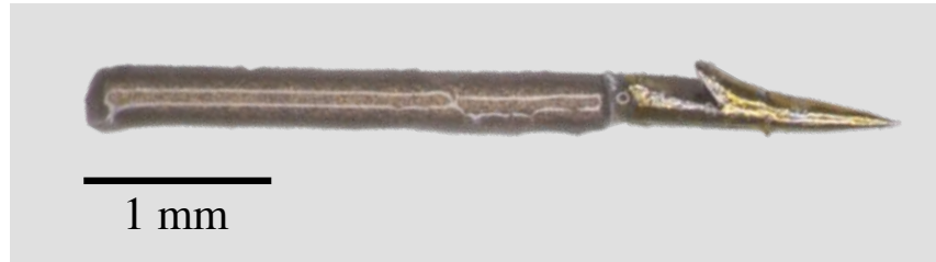
Figure 4.17: Magnetic microrobot for floater removal consisting of a permanent cylindrical magnet and a hook.
