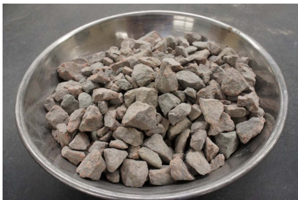
Fig. 2: Crushed granite used as coarse natural aggregate (NA) in concrete.
