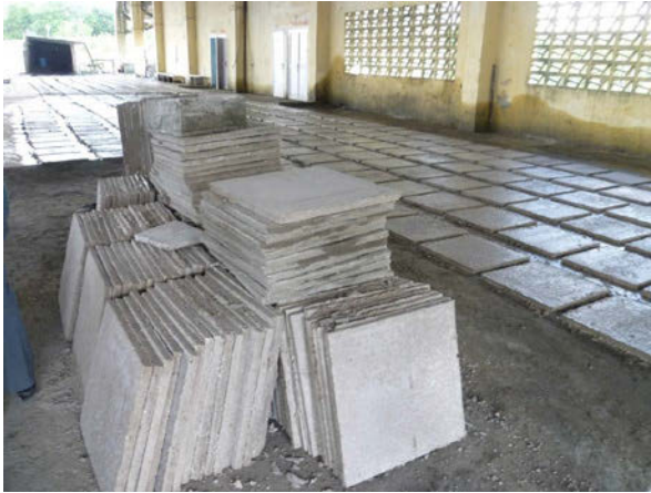
Fig. 4: Prefabricated elements with LC 3 cement produced in Cuba, Siguaney a) hollow concretes blocks b) hydraulic tiles (courtesy of F. Martirena)
