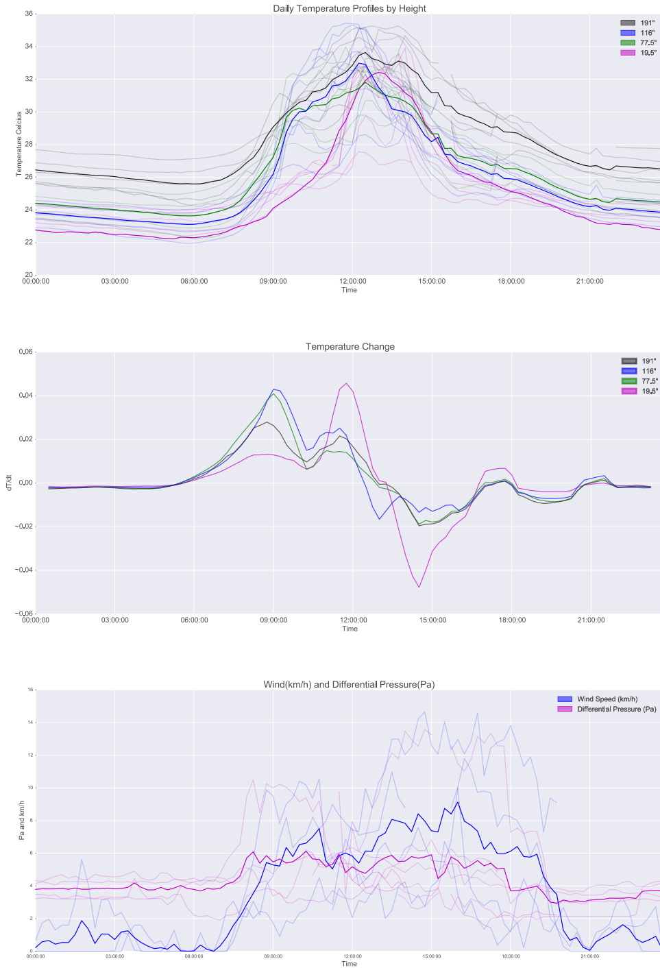
Fig. 7: (a – top) Daily temperature profiles and averages (opaque lines) for spring-time operation of the DSF at varying heights; (b – middle) Time derivative of temperature change throughout the day at each height; (c – bottom) wind and differential pressure averages for the DSF.
