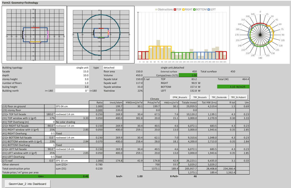
Fig. 3: Input parameters and graphical representation of obstructions in Form2.
