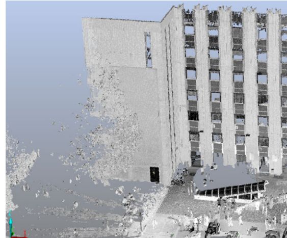
Fig. 9: Point cloud image from laser scanning relief.
