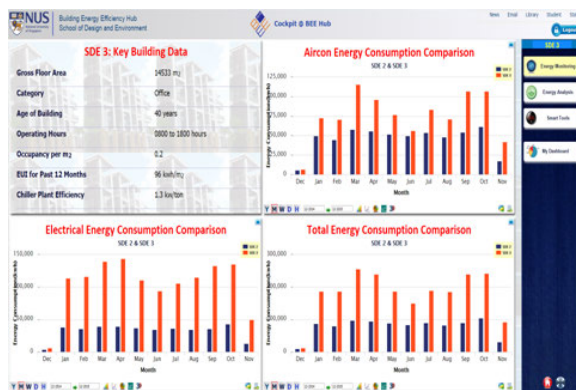
Fig 4: Energy monitoring and comparison between buildings.
