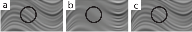
Figure 48: Discretizations of the gradient. (a) Full 3 \times 3 stencil. (b) Forward and backward differences. (c) Central differences.
