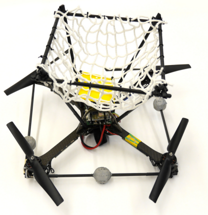
Figure 1.6. A quadcopter with attached catching net, as used to demonstrate the algorithm. The centre of the net is mounted above the vehicle’s centre of mass in the quadcopter’s e_3 direction.
