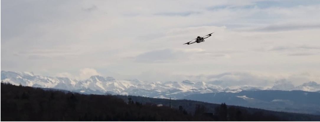
Figure 2.4 A quadcopter being flown by hand on the Züriberg after the simulated complete failure of one propeller. This is a still taken from the video at www.mwm.im/1/VidFailsafe2 .
