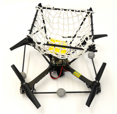
Figure 2.1 To validate the method of [P1], a quadcopter with an attached net is tasked to catch a ball thrown by a person.
