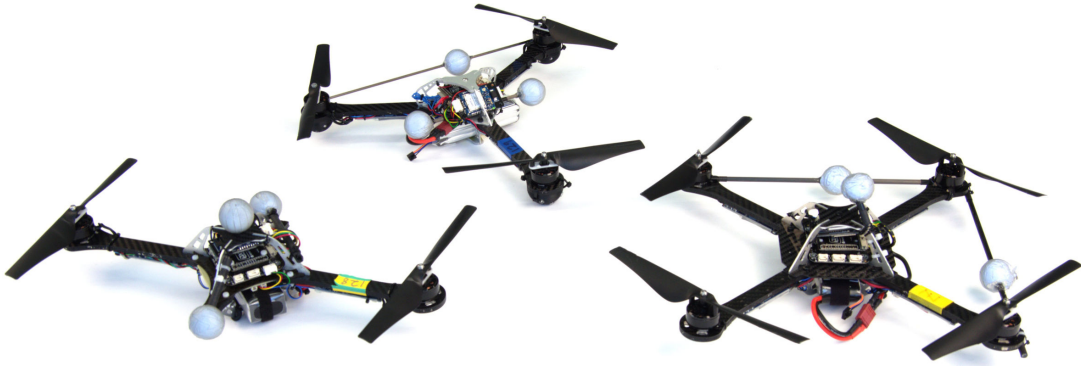
Figure 3.11. A novel class of flying vehicles, from left to right: bispinner, trispinner, and quadspinner. For each vehicle, all propellers rotate in the same direction, causing the vehicle to rotate in the opposite direction in hover. Extension 2 contains a video showing each of these vehicles flying.
