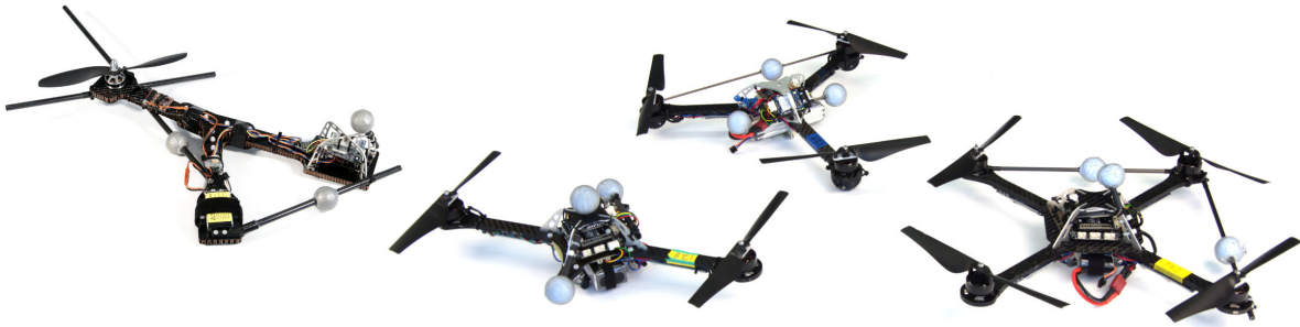
Figure 2.2 Novel flying vehicles developed in this thesis,, from left to right: the mono-, bi-, tri-, and quadspinner. The monospinner is described in [R2], the remainder in [P3].
