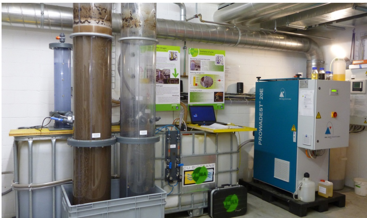
Figure 1: The nitrification reactor (left column) and distiller (right) at Eawag (Photo: B. Etter).
