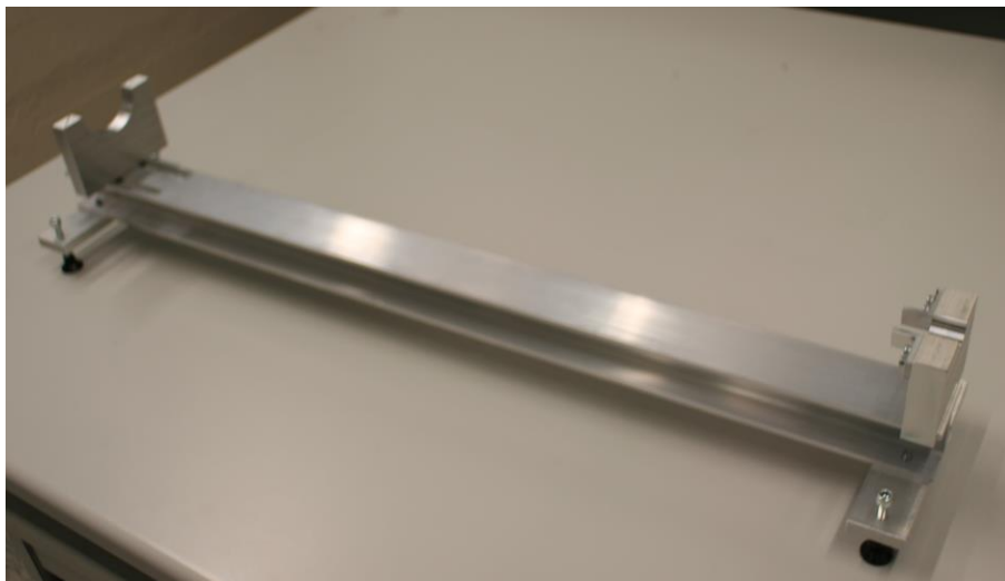
Figure 50. (a) Jig for IMU initialization.
