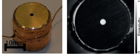
Figure 6.3: Emissivity calculation. Left) Picture of the used metallic cylinder with a deep hole which acts as a black body cavity and the surface coated with gold to obtain similar emission properties to our sample. right) Emissivity map calculated with the camera software.
