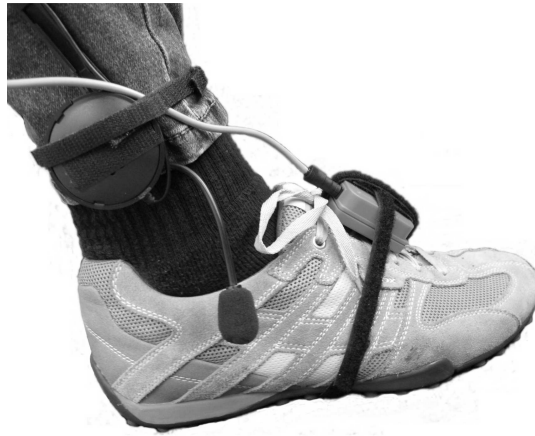
Figure 8: Sensor setup and microphone attached to the ankle
