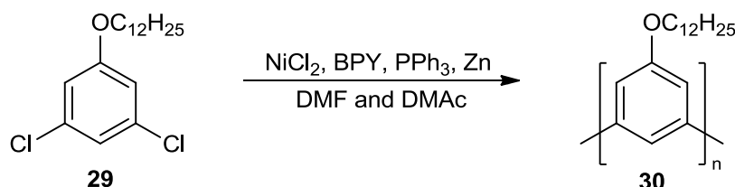
Scheme 8. Synthesis of PMP 30 by Ni-catalyzed homocoupling. BPY: 2,2'-Bipyridine.
