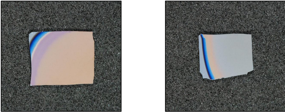
Figure 105: Heat treated samples (\text{Au}96\text{Pt}4)\text{Al}_2 and (\text{Au}57\text{Pt}43)\text{Al}_2 , with a thickness gradient introduced by polishing away part of the surface. In both samples differently coloured layers appear, before the substrate (blue) becomes visible.
