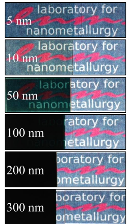
Figure 19: Images of thin Au films (left part), in counter light. After a thickness of 100 nm is reached, the films are opaque.
