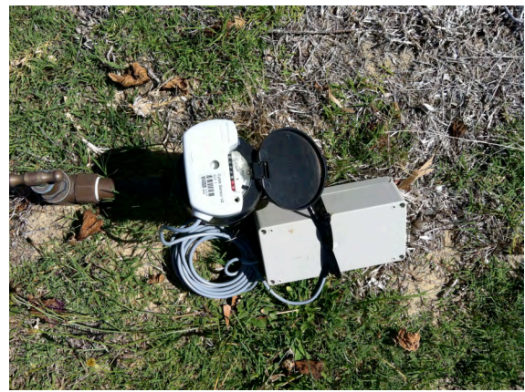
Figure 5: A Unidata logger and transmitter is connected to this Actaris water meter via a Cyble sensor
