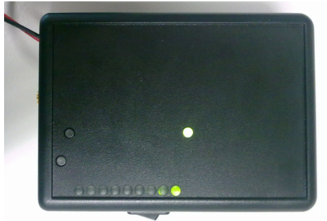
Figure 4.23. Top view of the case with the LEDs indicating the chosen modulation frequency f_{mod} .
