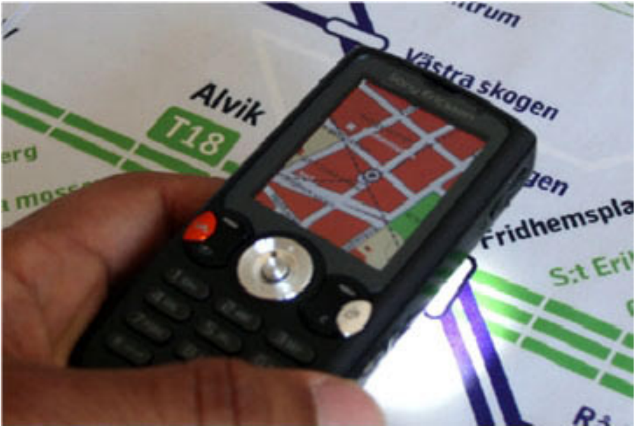
Fig. 3. Outside-in approach tracking the phone light source and streaming the data to the phone. The spatially aware device augments a physical map with a detailed interactive road map of the area of interest [29].
