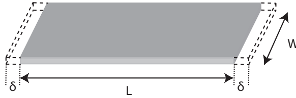
Figure 62: Magnetostrictive sensor made of ferromagnetic alloy ribbon 2826MB from Metglas, Inc. Dimensions of sensor 3 mm x 2 mm x 30 \mu m. Length change of 2\delta due to magnetostriction.
