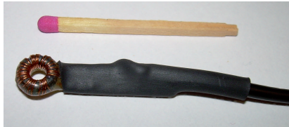
Fig. 5.6: Constructed AC current transformer with a sensitivity of 100 mV/A to measure the drain source current I_{DS} of the MOSFET.
