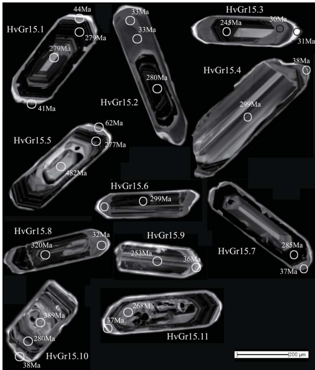
Figure H.2: CL-imaging of analysed zircon grains in sample HvGr15 showing the location of the spot analyses and the calculated age (uncorrected)
