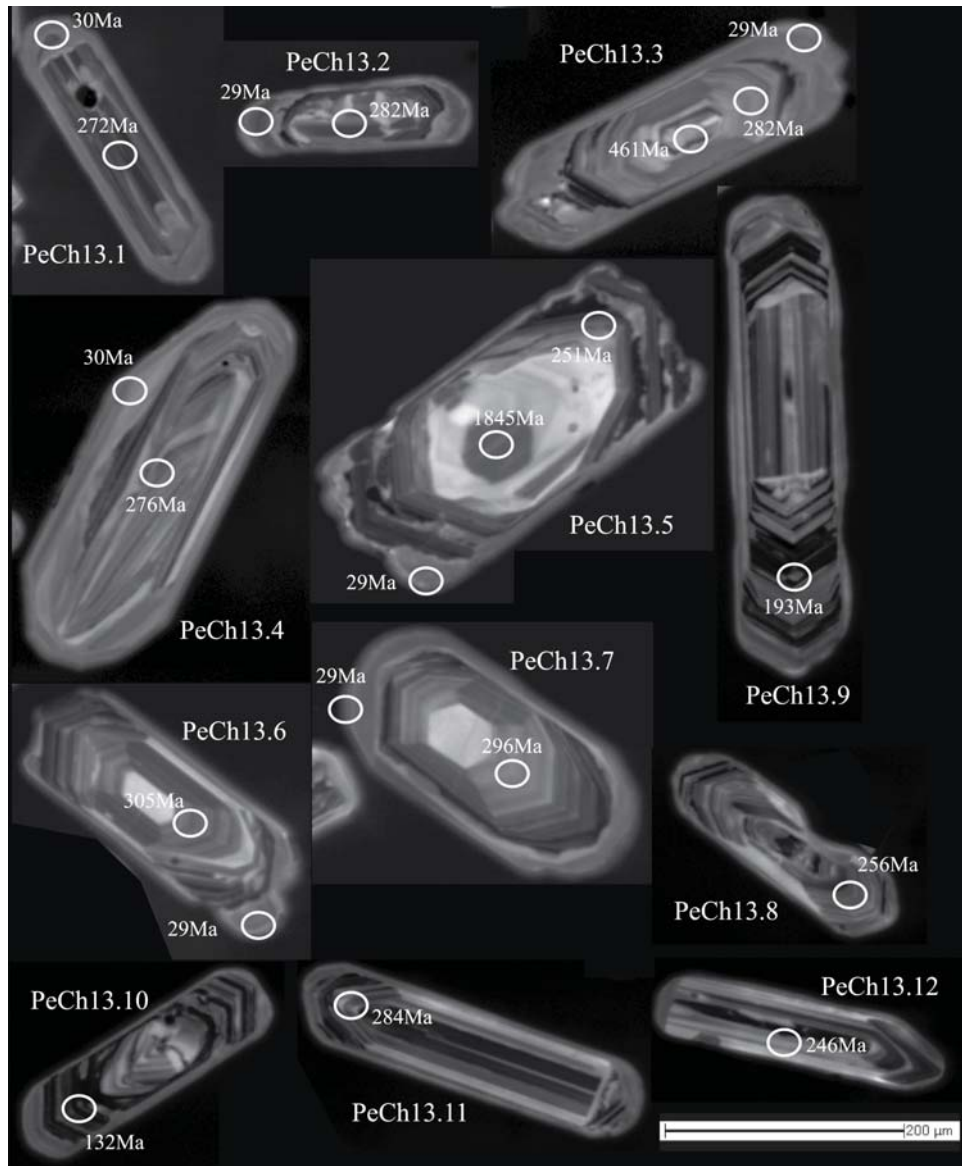
Figure H.9: CL-imaging of analysed zircon grains in sample PeCh13 showing the location of the spot analyses and the calculated age (uncorrected)
