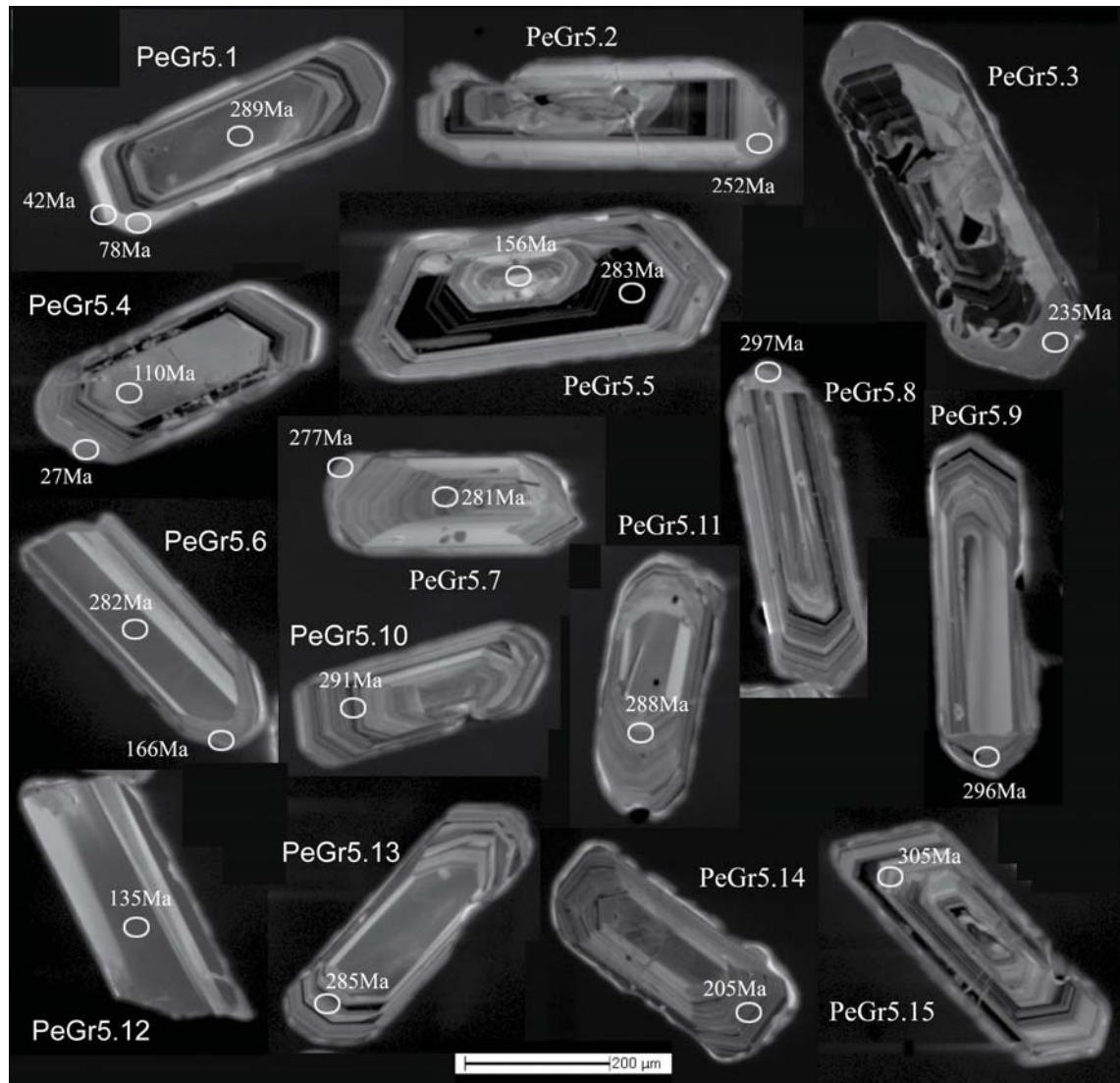
Figure H.1: CL-imaging of analysed zircon grains in sample PeGr5 showing the location of the spot analyses and the calculated age (uncorrected)
