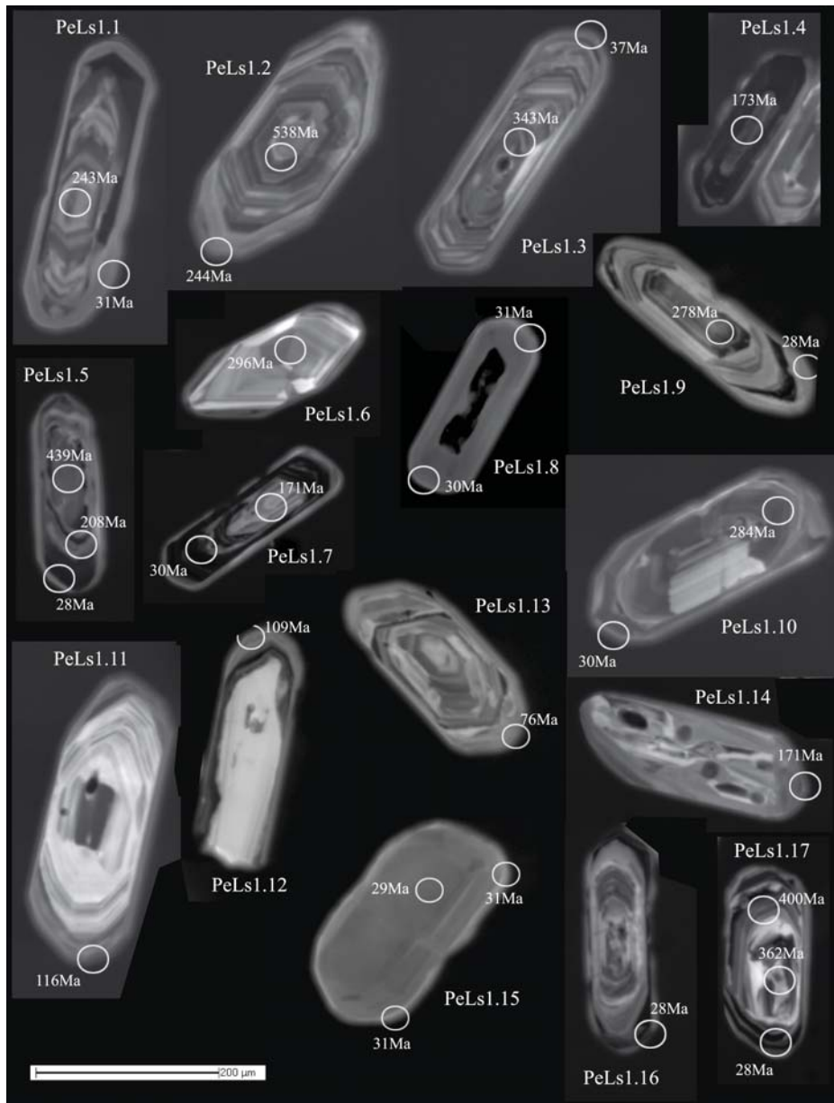
Figure H.13: CL-imaging of analysed zircon grains in sample PeLs1 showing the location of the spot analyses and the calculated age (uncorrected)
