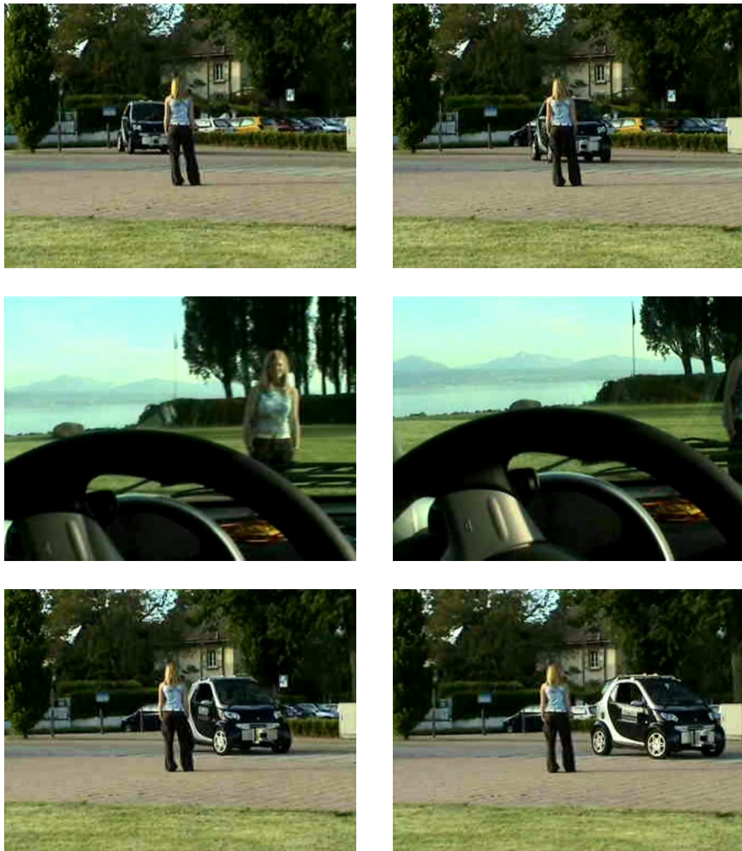
Figure 3.26: An experimental snapshot sequence of the testing vehicle with the probabilistic reactive obstacle avoider. The vehicle is steering away from sectors of occupied angular clearance map (pedestrian and static environmental objects).
