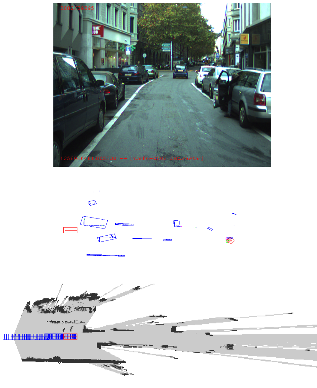
Figure 5.22: Detection of a vehicle moving away I (top: scene view, middle: extracted objects, bottom: occupancy map).
