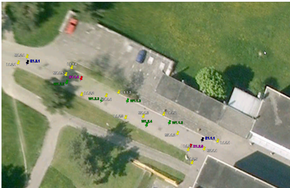
Figure 6.4: A section of the lane definition map based on global GPS coordinates. The L labelled points define the outer lane boundaries, whereas the M labelled points define the middle of the road. Other GPS points are the waypoints defined by the RNDF description.
