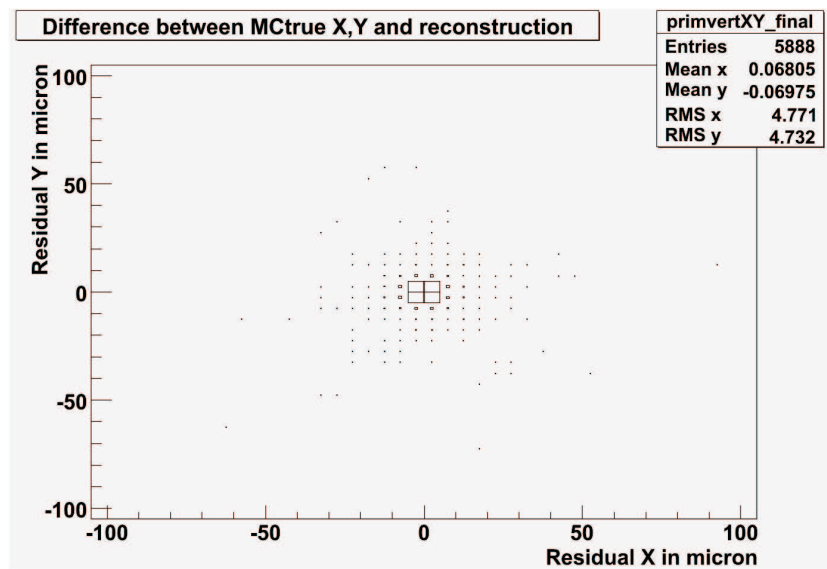
Figure 5.2: Reconstructed position in X , Y of the primary vertex w.r.t. the MC truth position of the \nu -interaction in the charm-CC MC sample after the decay search procedure and eye-checks were applied.
