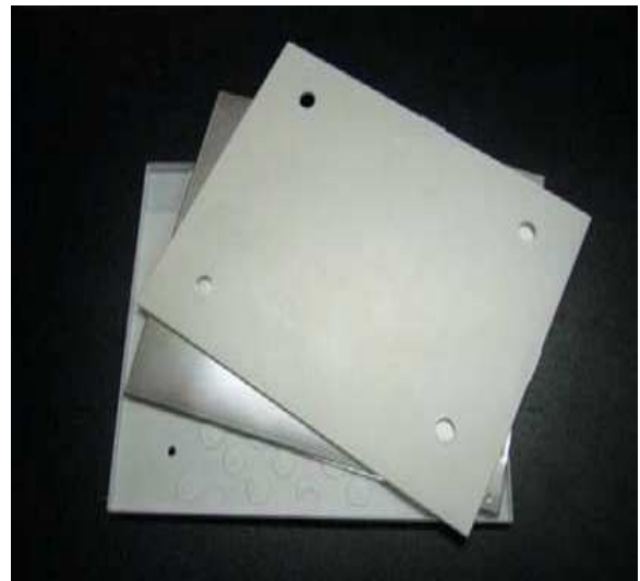
Figure 3.18: Opened plastic CS box of the OPERA ECC cell, with the two emulsion layers packed in an envelope. Picture from [207].
