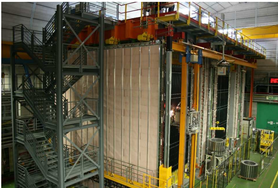
Figure 3.13: Picture of the OPERA detector. The beam is entering from the left. The Veto is the white plane behind the staircase.
