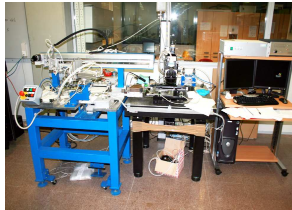
Figure 3.37: Oil emulsion plate changer, here the prototype at LNGS.
