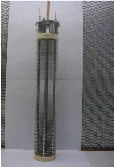
Figure 2.12: View of the muon monitor without its stainless steel casing, its height is 60 cm. Picture from [204].
