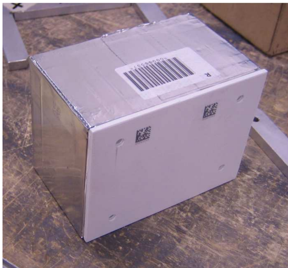
Figure 3.17: The OPERA Brick with CS-box. To identify the brick a matrix code is printed on it. The dimensions are 12.8 \times 10.2 \times 7.9 \text{ cm}^3
