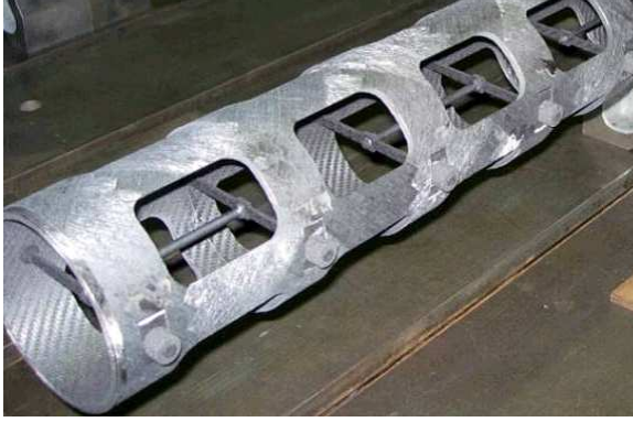
Figure 2.6: View of the CNGS graphite target. Picture from [207].
