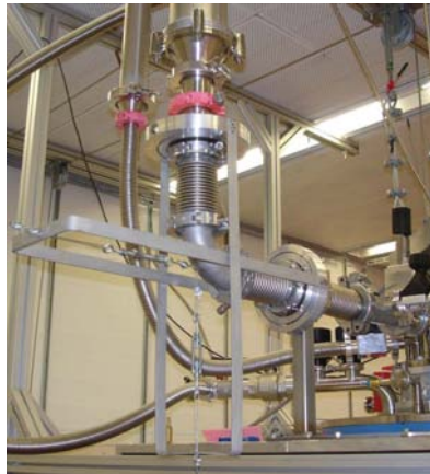
Figure A.2: Double gimbal vibration isolation. The pumping side (top) is connected to the cryostat still line (right) using two flexible stainless steel bellows. The bellows are elongated to their nominal length using steel ropes suspended at two gimbals. The two gimbals are fixed at two rings which are free to pivot around one axis relative to the two inner rings. The inner rings themselves are also free to pivot about the orthogonal axis. The connections were implemented with a set of 16 tight fitted axial deep groove ball bearings.
