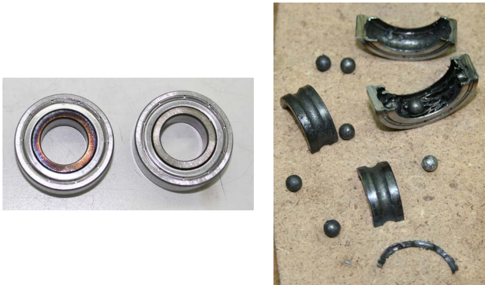
Fig. 5.62 Failed Bearings after Disassembling: a) Contact Surface b) Bearings from inside.
