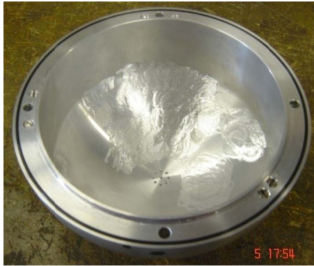
Fig. 5.37 Cone grinded from Inside at Location of the Balancing Plane 2 and drilled at Location of Balancing Plane 1.
