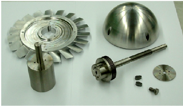
Fig. 5.44 Individual Parts of the Rotor-Shaft Assembly.
