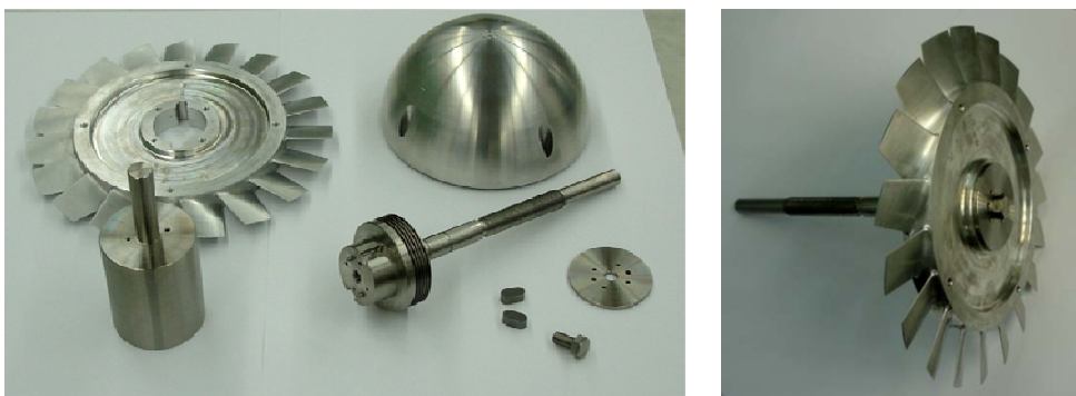
Fig. 5.23 a) Individual Parts of the Shaft-Rotor Assembly b) Shaft Rotor Assembly.
