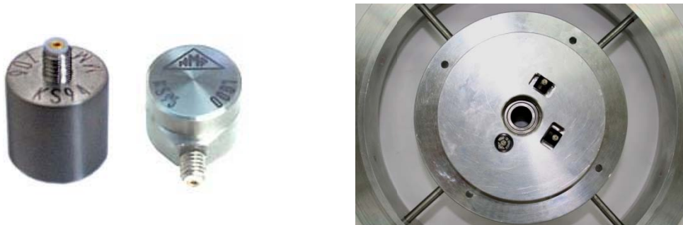
Fig. 5.52 a) Accelerometer KS-94/95B.10. b) Accelerometer Mounting Arrangement.
