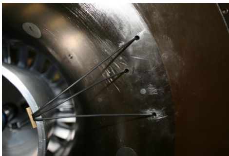
Fig. 5.55 The Three Cables are lead along the Hub and fed through existing Holes in the Impeller Shroud.
