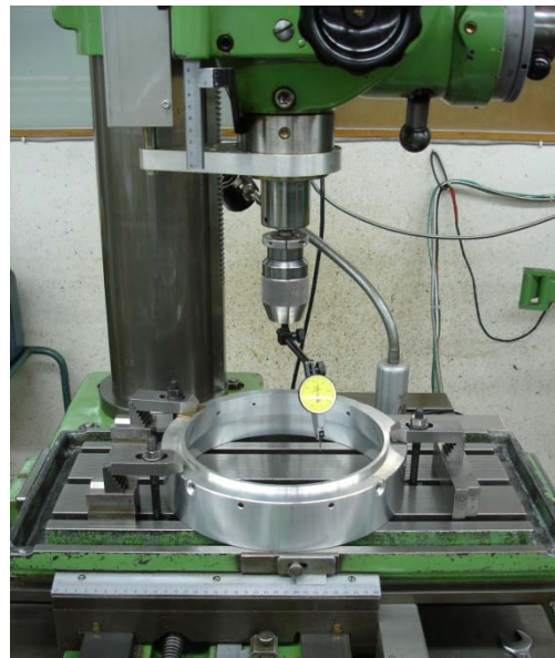
Fig. 5.42 Stator Outer Ring mounted on a Drilling Machine for Alignment.
