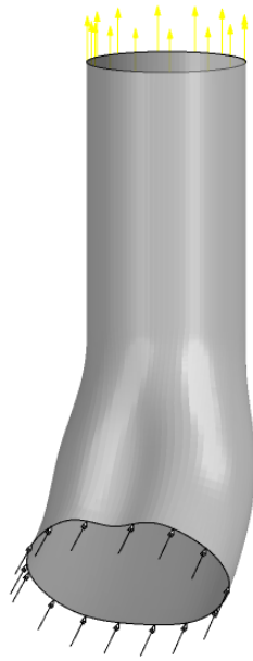
Fig. 3.18 Final optimized Compressor Inlet Duct Topology: Kidney-shaped.
