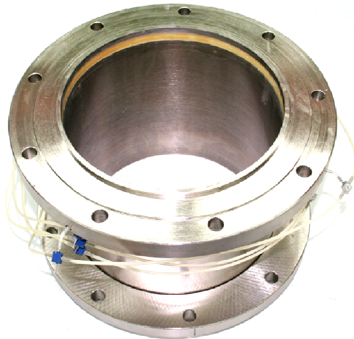
Fig. 5.60 Successful Integration of an Abradable Wax Layer into the Rotor Casing.
