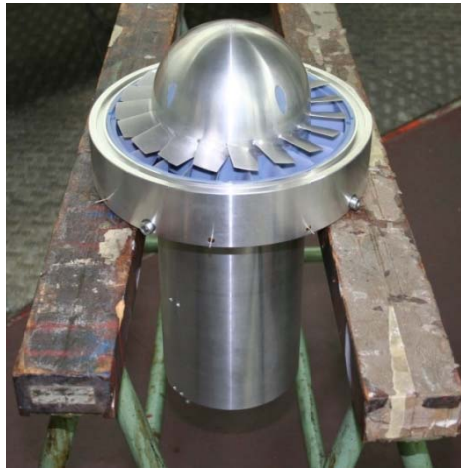
Fig. 5.46 Ready to be integrated: Axial Compressor Assembly.
