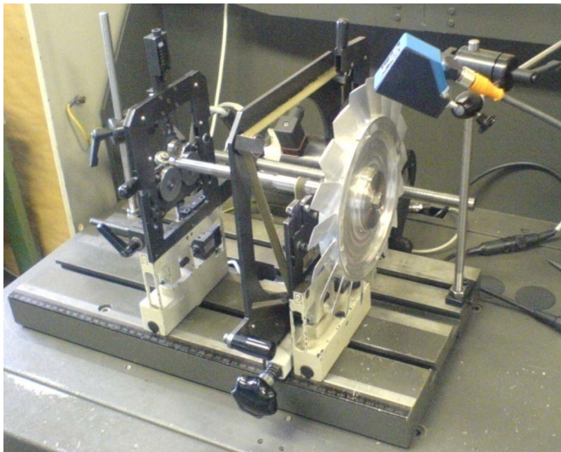
Fig. 5.35 Rotor-Shaft Assembly being balanced on a Schenck HS 10/CAB 690 Balancing System.
