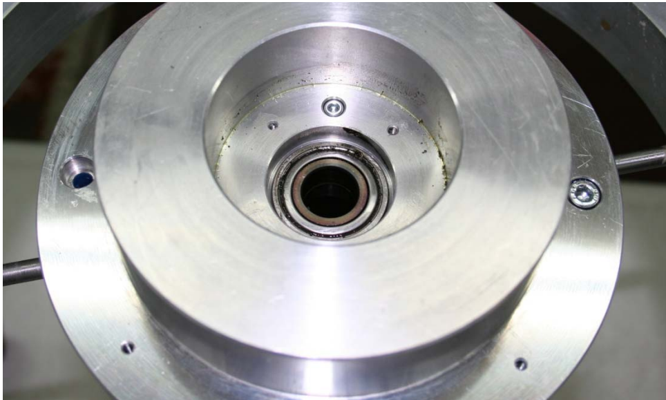
Fig. 5.61 The failed Bearings still inside the Stator Inner Ring.
