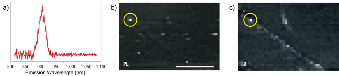
Figure 4.6: Observation of localized PL from a negatively charged defect by Indhira O. Maciel et al. [63]. a) Photoluminescence emission from the emissive spot. The nanotube chirality is attributed to be (9,1). Note the slight blue detuning of the PL (central emission at 904 nm) compared to the expected emission wavelength of 912 nm for a (9,1) SWNT. b) Near-field photoluminescence image of the SWNT revealing localized excitonic emission. The scale bar denotes 250 nm. c) Near-field Raman imaging of the same SWNT, where the image contrast is provided by spectrally integrating over the defect-induced D bands. Independent analysis of the high energy G' raman peak reveals that the defect is negatively charged.
