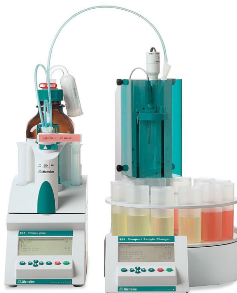
Figure 6.3: Titration device of manufacturer Metrohm equipped with a fully automatic sample changer
