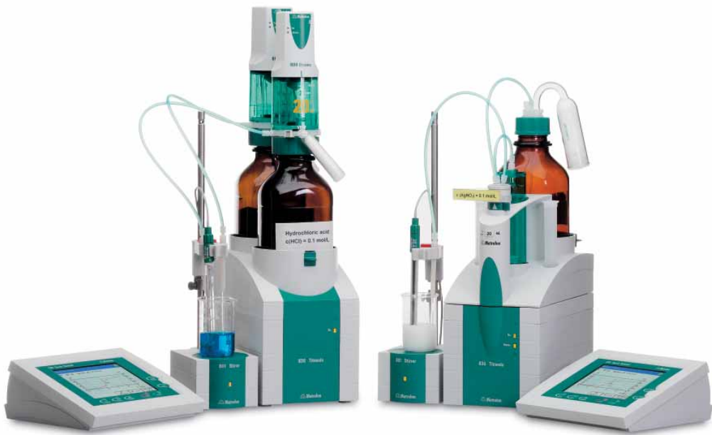
Figure 4.2: State-of-the-art titration devices from the manufacturer Metrohm
