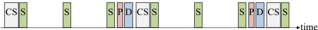
Figure 8.1: A slot assignment on a sensor node with 4 tasks: Periodically sample a sensor [S], process the sensor data [P], disseminate the processed data [D], and run a clock synchronization algorithm [CS].
