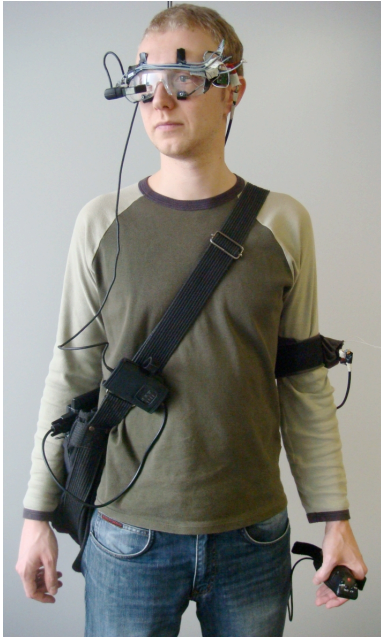
Figure 5. Person using the wearable EOG goggles together with a head-up display (HUD) and a wearable keyboard (Twiddler2) for interaction in a mobile setting.
