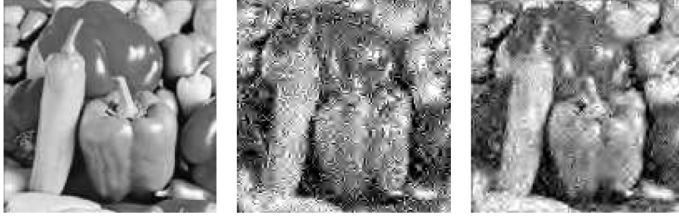
Figure 5.1: Example performance of model based and standard CoSaMP recovery. From left to right, the original image with n = 128 \times 128 = 16,384 pixels and the images recovered using m = 5,000 measurements from the standard CoSaMP algorithm (middle) and the model based recovery (right). Taken from (Baraniuk, Cevher, Duarte, and Hegde 2008, Fig. 5).
