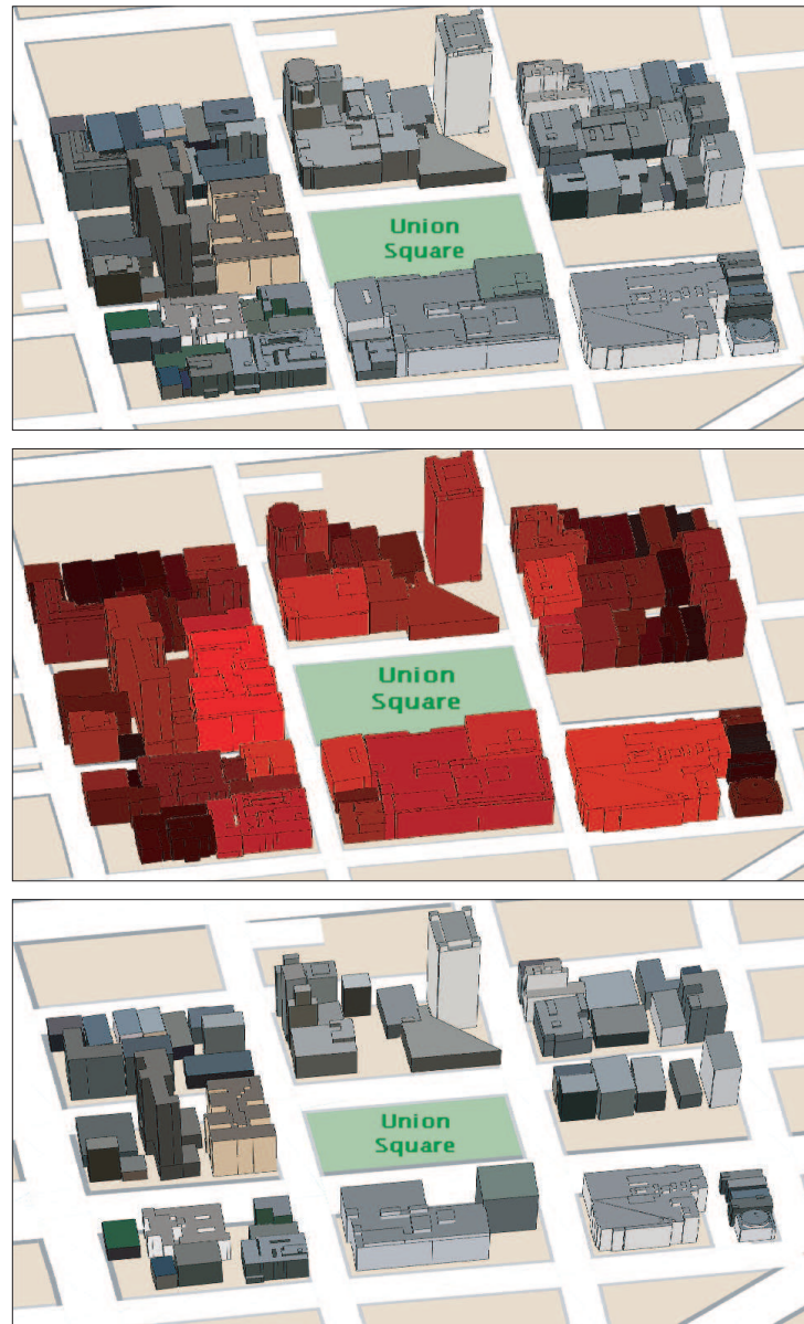
Figure 5.9: Generalization. (Top) Original block. (Middle) Importance scores for the buildings, where the red saturation of a building is proportional to its importance. (Bottom) Generalized blocks.
