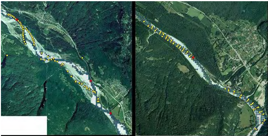
Fig. 6.12: Example for horizontal (left) and vertical (right) deviations between DTM and field measurements. Orthophoto is from 2000, river bed topography left from 2002, and 1996 on the right. Yellow (big) dots: geodetic field measurements in 2005, blue (small) dots: simulations under low flow conditions using the underlying river bed topography. On the right sight, the horizontal coherence is good, but there are vertical differences between the DTM and field measurements of approx. 1.5–2 m.
