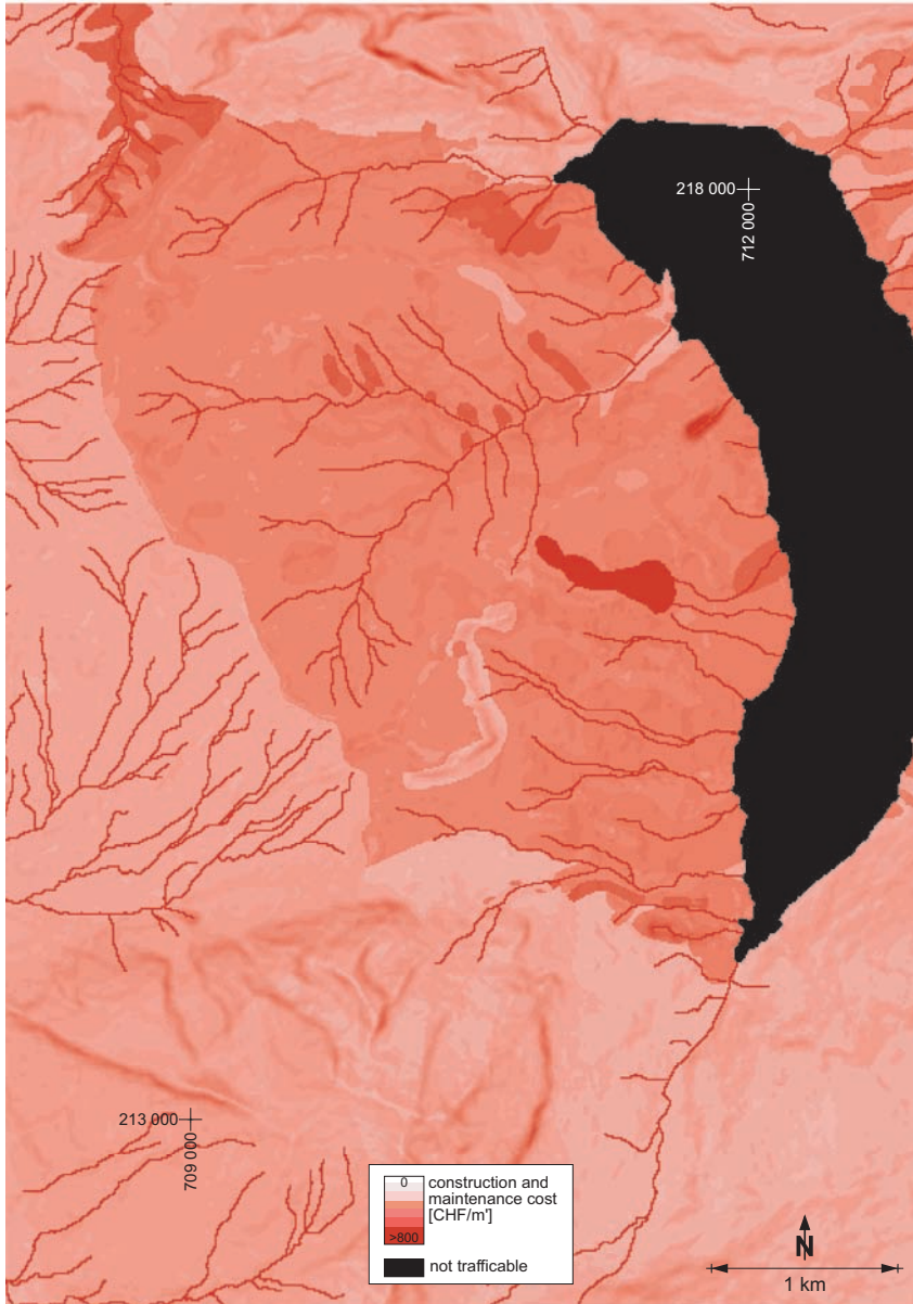
Figure 1.7: Spatial variability in road life cycle costs for Scenario III, based on slope gradient and geotechnical soil properties. The lake “Wägital” is at eastern boundary and watershed is at western boundary. (5 km × 7 km)
