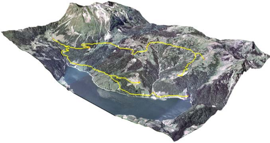
Figure 4.18: Cost-optimal road network (Alternative C!) indicated in yellow (length = 20.9 km). Area (5 km × 7 km) at Wägital, Switzerland
