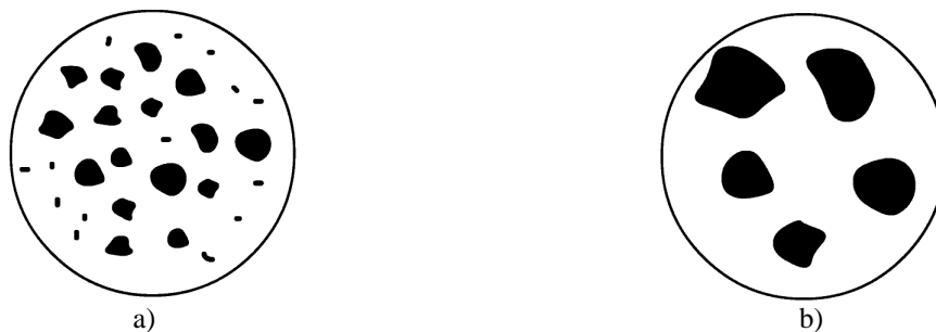
Fig 4.8 Model of contact area, different asperity contact geometry and distribution; a) rough; b) smooth surface
