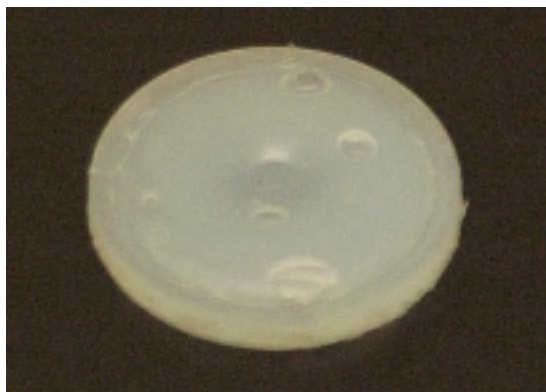
Fig 4.1 PFA toroid with some bubbles, diameter 30 mm
