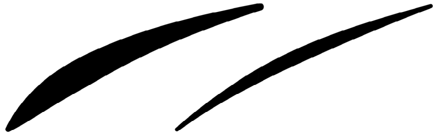
Figure 3.2-1: Deverson baseline blade and real engine blade
