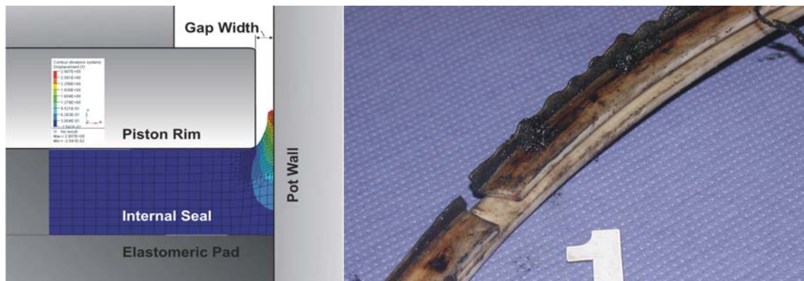
Figure 1 Principle deformation of the FE-mesh compared to a real bulge of an internal seal
