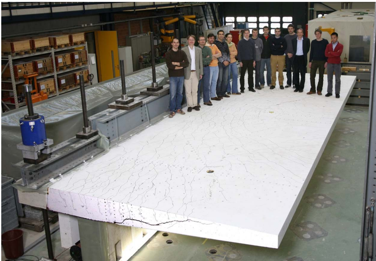
Figure 1: Full scale model of bridge deck cantilever (10.0 m length, 4.2 m width and 0.38 m maximal thickness)
