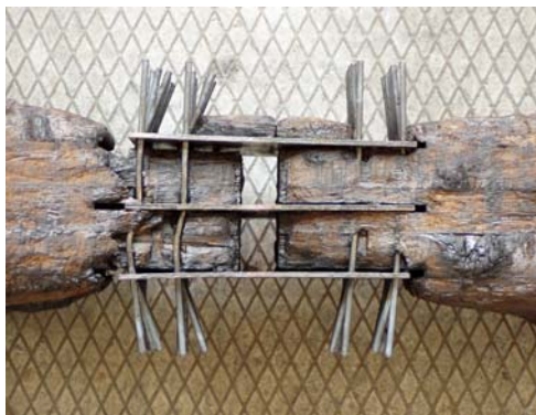
Figure 1 Multiple shear steel-to-timber connection after fire test (left) and charring model for unprotected (line 1) and protected (line 2) timber member (right) according to EN 1995-1-2
