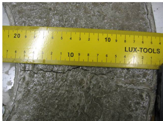
Figure 2 Crack on ring specimen
