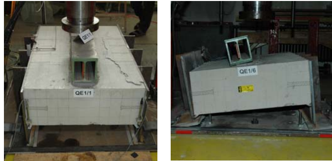
Figure 3 Failure modes concrete outbreak and shearing of the studs
