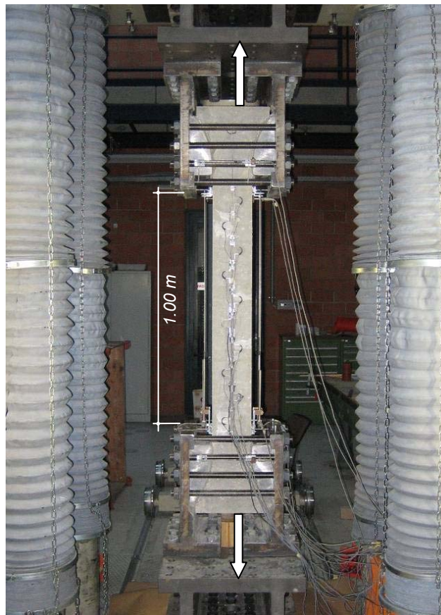
Figure 1 Test setup for full scale UHPFC tensile members with ordinary reinforcement and a measurement length of 1.00 meter.
