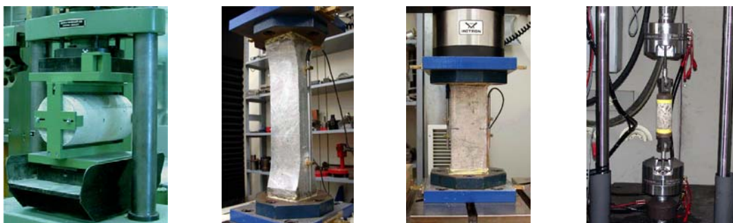
Figure 1 Centering device for splitting tension tests (left). Setup of the uniaxial tension tests on unnotched and notched prisms (centre) and on cores (right)
