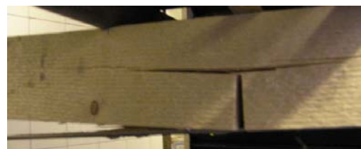
Figure 3 Failure by the bending test
