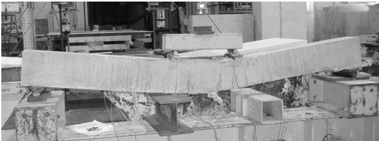
Figure 1 Two point flexural test on a corroded beam
