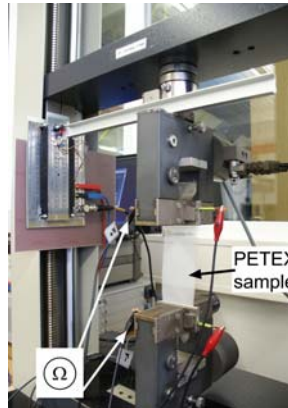
Figure 3.60: Tensile test setup. The resistance of the copper wires in PETEX is monitored during the tensile tests.
