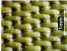
Figure 3.20: Acryl-cotton substrate for screen-printing
