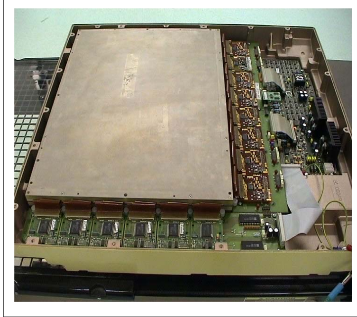
Figure 2.1 A photograph of the amorphous silicon based detection unit (IDU) of the PortalVision™ aS500. The IDU consists of 1024 \times 764 pixels with a pixel pitch of 392 \mu\text{m} resulting in a total area of 40 \times 30 \text{ cm}^2 . Next to the sensor, electronics is required for the acquisition of a portal image.
