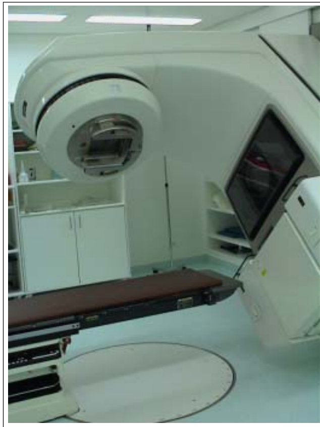
Figure 1.1 During the irradiation, the patient is lying on the couch under the treatment machine (gantry). High-energy photons are generated by bremsstrahlung within a target. In order to irradiate the tumor from different beam directions, the gantry can be rotated.
