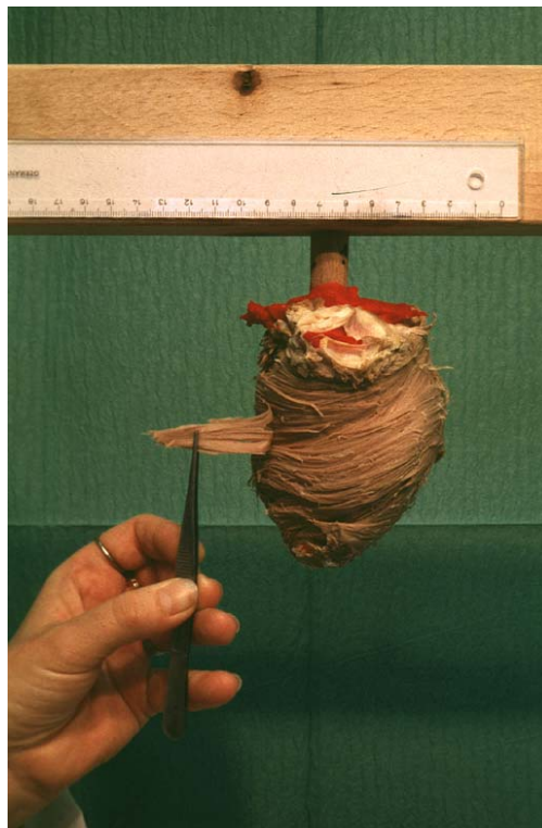
Figure 2.10 Fibre strand peel-off technique (Lunkenheimer et al. )
