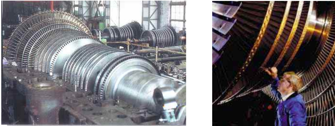
Fig. 1.-1 High and mid pressure steam turbines with shrouded blades
