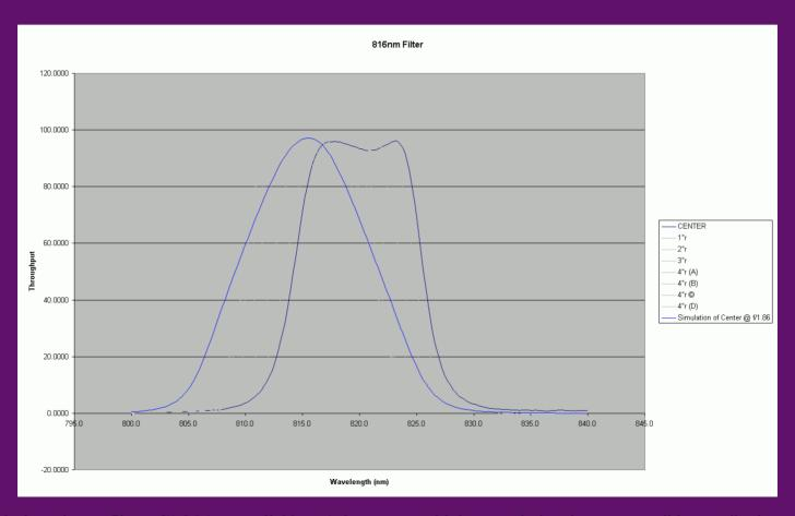
Broader filter and triangular profile at f/1.86 (vs. parallel beam) decrease sensitivity to emission, increase possible contribution of nightsky lines
