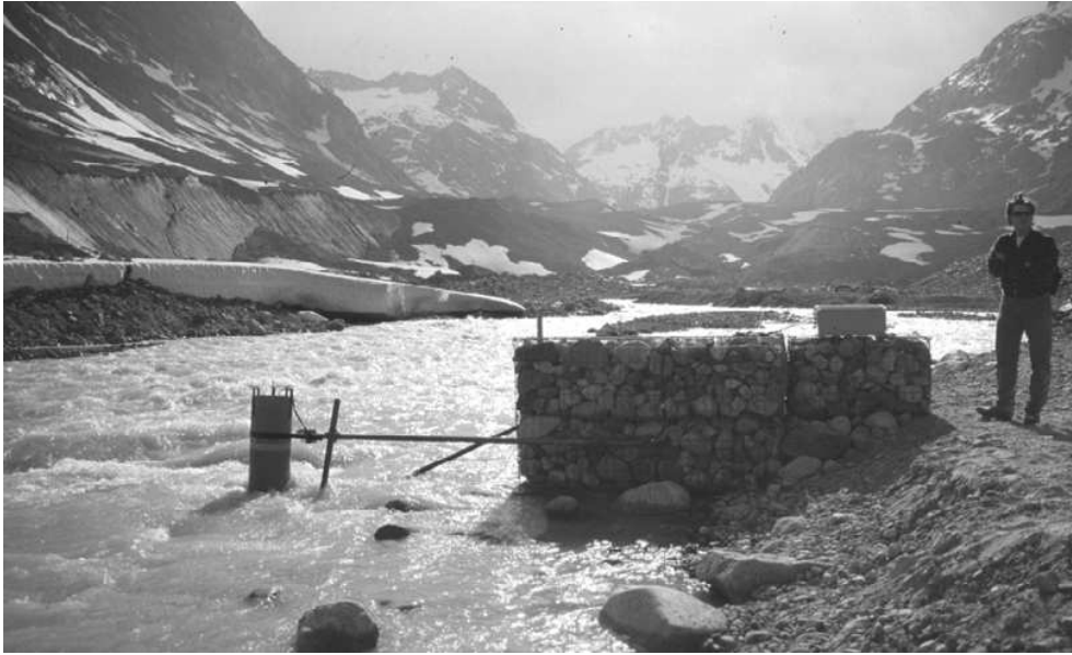
Figure 3.8: The gauging station in June 1999. The terminus of Unteraargletscher can be seen in the background (photograph taken by T. Schuler).
