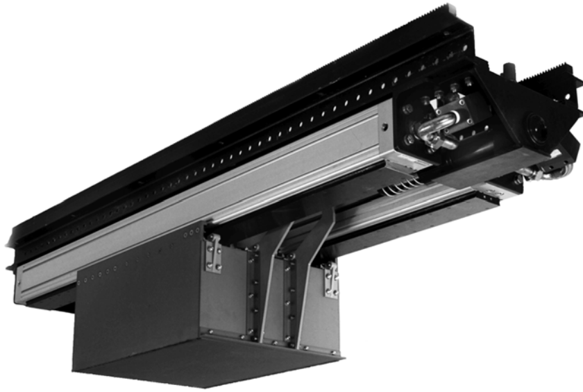
Figure 3.5 Pneumatic slide acceleration mechanism with the two double acting pneumatic linear drives, the plain bearing guides, the slide box and the pneumatic cylinder driven flap opening mechanism, prior to installation into the framework on the hill slope ramp.
