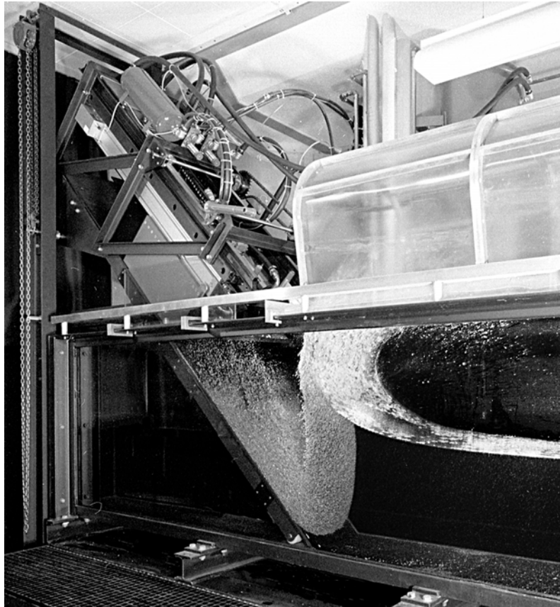
Figure 3.7 Slide impact experiment at F = 2.0 , m = 108 kg, h = 0.45 m and \alpha = 45^\circ after slide release with the slide box in the end position.
