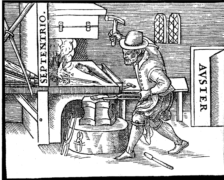
An illustration showing how hot iron, when beaten, can be made magnetic, from Gilbert's book De Magnete , (1600).
