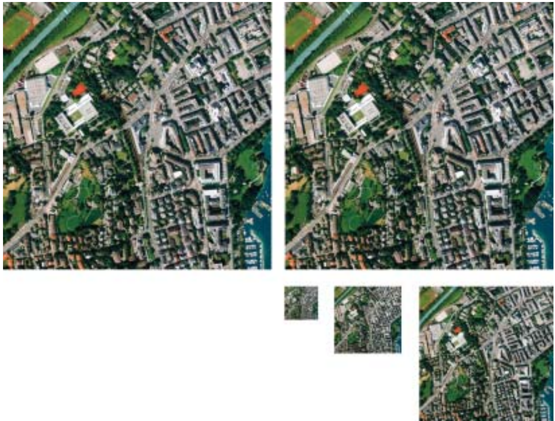
Fig. 38: Progressively loaded PGF ortho-photo (the four images in the right half) and its original bitmap (top left image). The compression ratio is 1:7.
