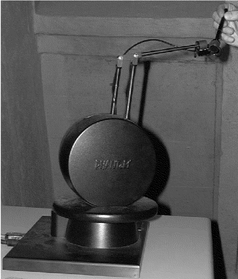
Figure 1.10: The unmodified PHANToM force-feedback device
