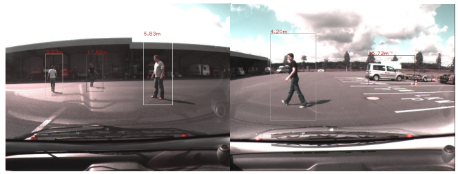
Fig. 3. Two images from parking lot dataset. Brighter rectangles indicate a high detection probability. On the left: multiple pedestrian detection is shown with different level of detection probability. On the right: a car is detected as a pedestrian with very low confidence due to a false positive in one of the detectors. Pedestrian distances are written in red.
