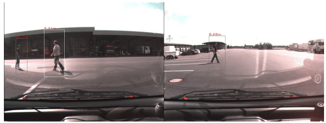
Fig. 4. Two images from parking lot dataset. Brighter rectangles indicate a high detection probability. On the left: the far away pedestrian receive a smaller vote with respect to the foreground person. On the right: a classic pedestrian crossing in simulated. Pedestrian distances are written in red.
